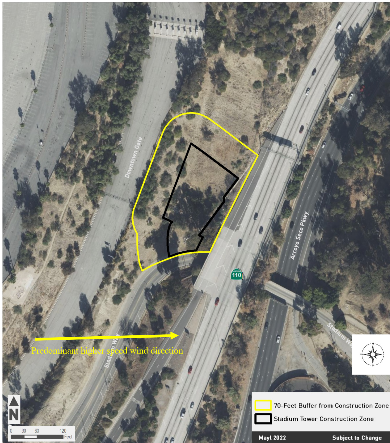
Figure 14: Stadium Tower construction site plan showing buffer zone of 70 feet, or to the nearest paved roadway
