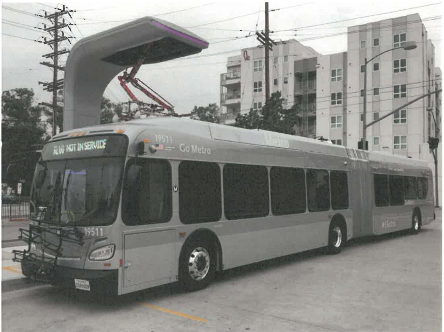
Metro New Flyer Electric bus charging in North Hollywood. All photos by Joe Linton/Streetsblog L.A.
