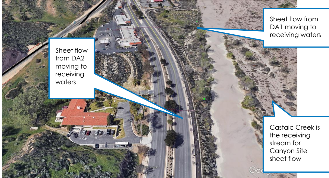
Figure 9: Canyon Siding Extension site DA2 drainage discharge location
