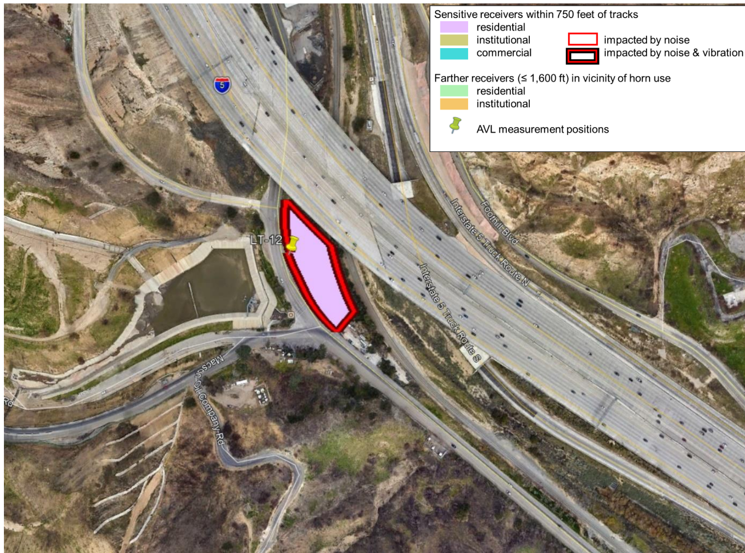
Figure 8: Construction Noise and Vibration Impacts in Vicinity of Balboa Double Track Extension in the City of Los Angeles
