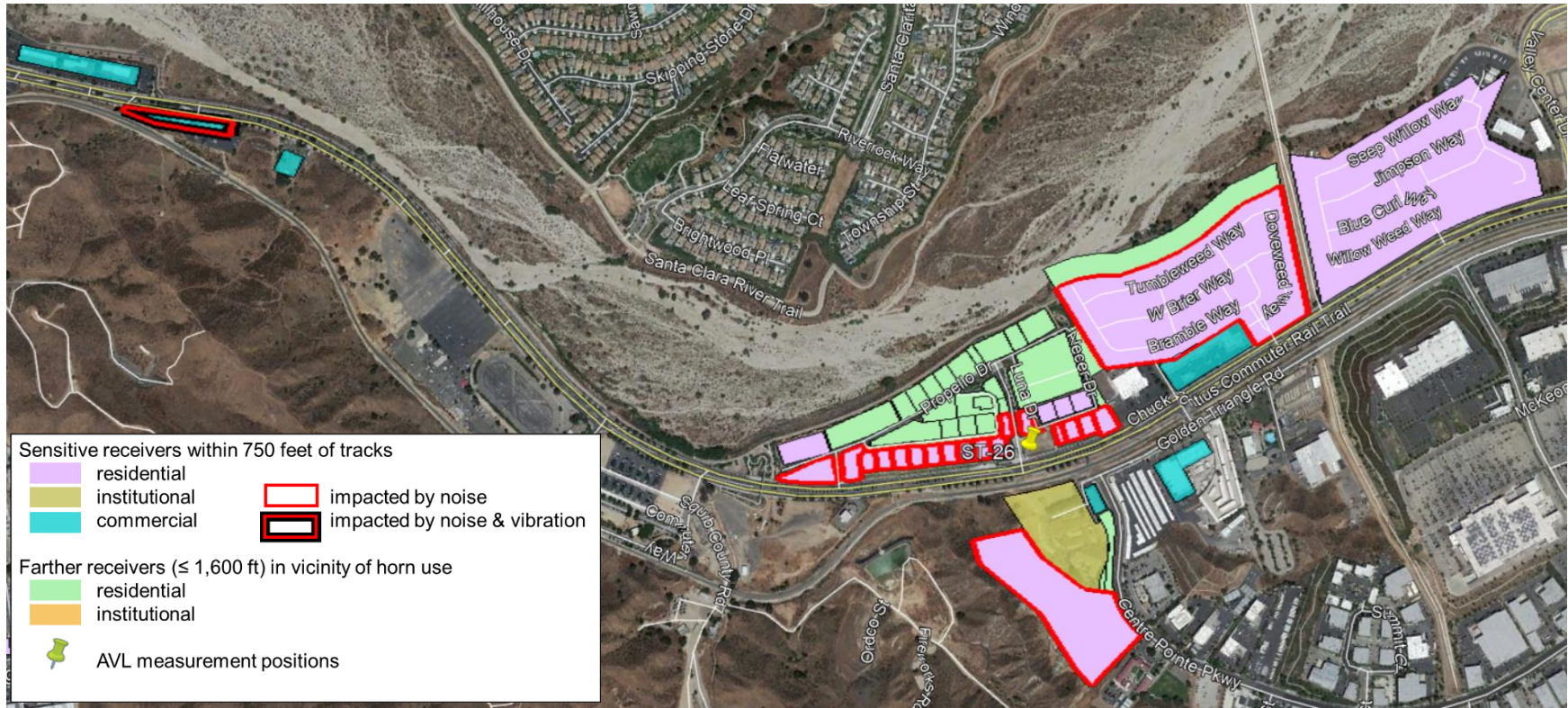
Figure 9: Construction Noise and Vibration Impacts in Vicinity of Canyon Siding Extension in the City of Santa Clarita
