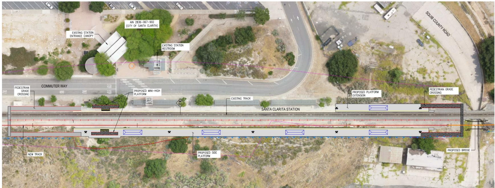
Figure 2-4: Canyon Siding Extension Proposed Station Platform Design
