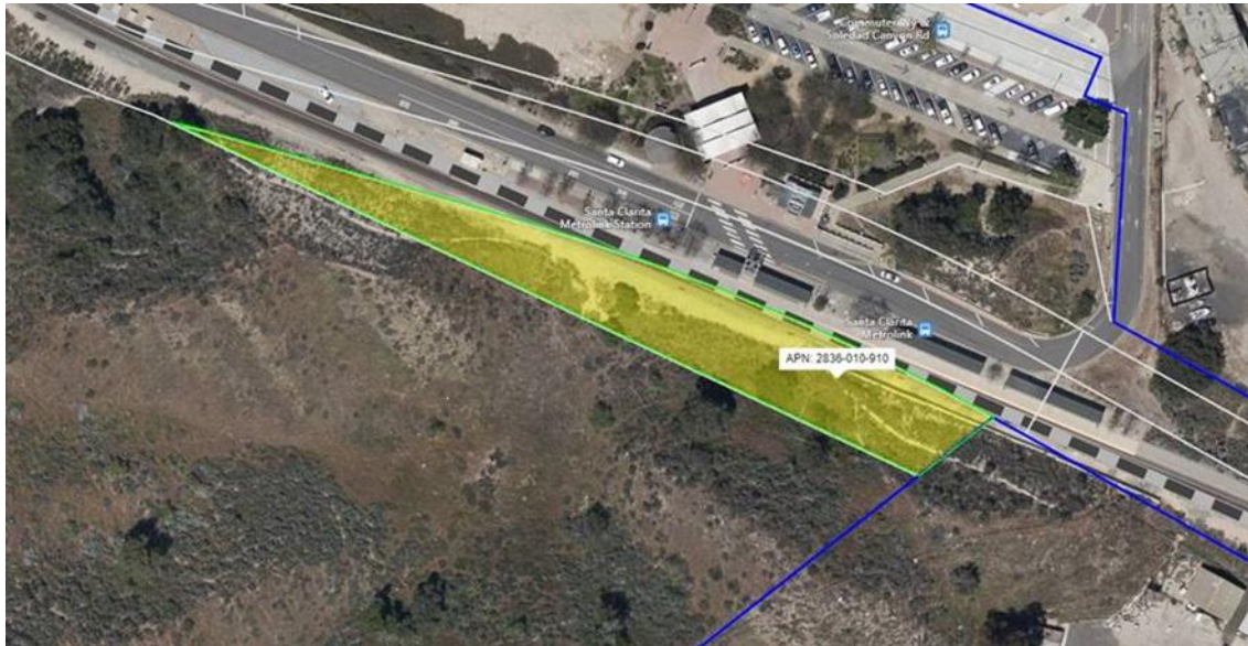
Figure 4.1: Santa Clarita Station Right-of-Way Impact
