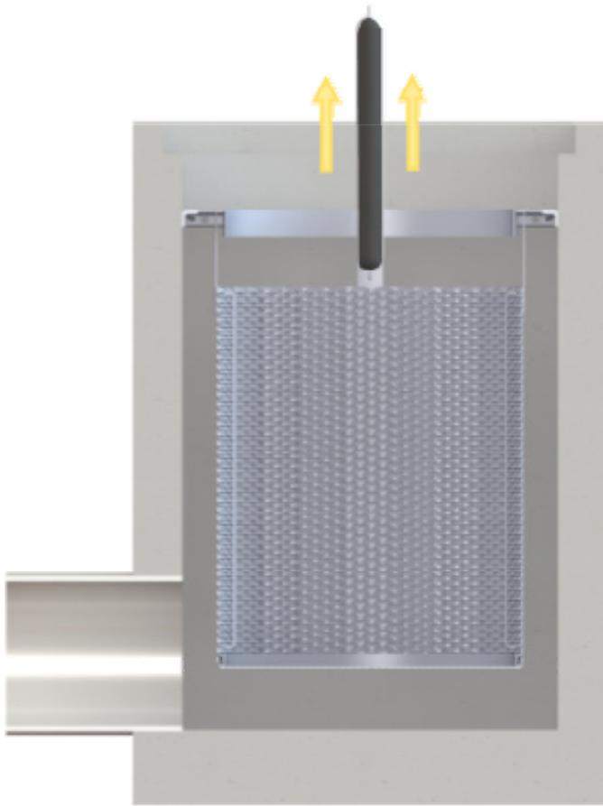
Remove the hydrocarbon boom that is attached to the inside of the filter basket. The hydrocarbon boom is fastened to rails on two opposite sides of the basket (vertical rails). Assess the color and condition of the boom using the following information in the next bullet point. If replacement is required install and fasten on a new hydrocarbon boom.
