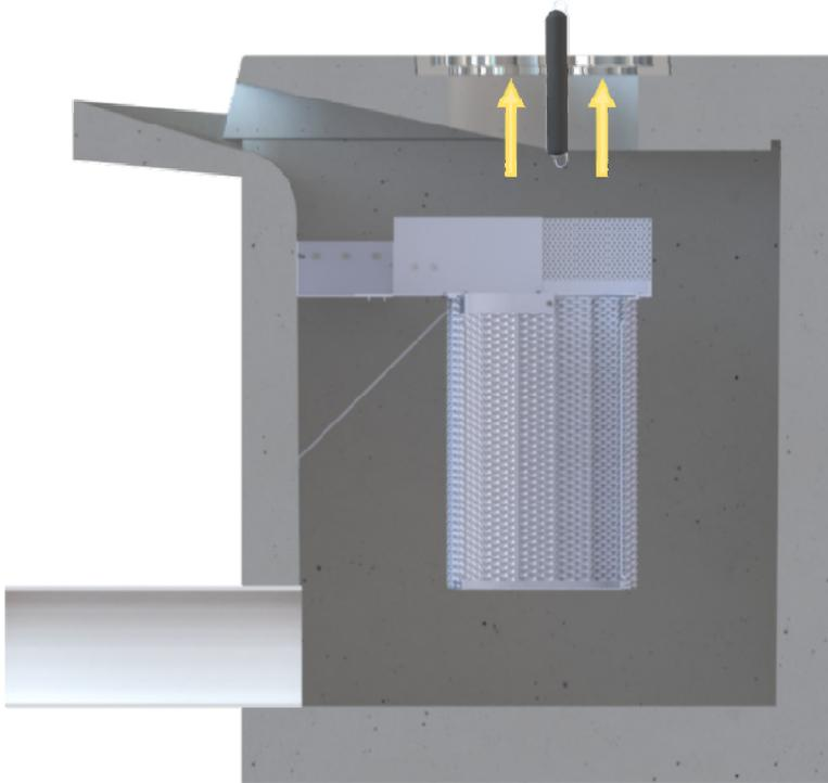
Remove the hydrocarbon boom that is attached to the inside of the filter basket. The hydrocarbon boom is fastened to rails on two opposite sides of the basket (vertical rails). Assess the color and condition of the boom using the following information in the next bullet point. If replacement is required install and fasten on a new hydrocarbon boom.
