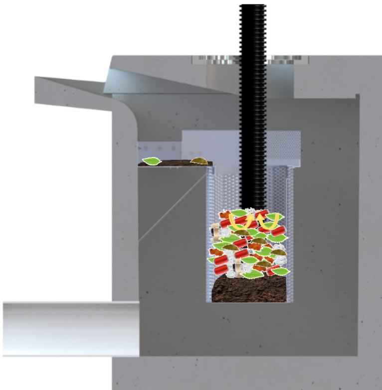
Insert the vacuum hose down into the filter basket and suck out debris. Use a pressure washer to assist in vacuum removal. Pressure wash off the weir and trough and vacuum out any remaining debris.
