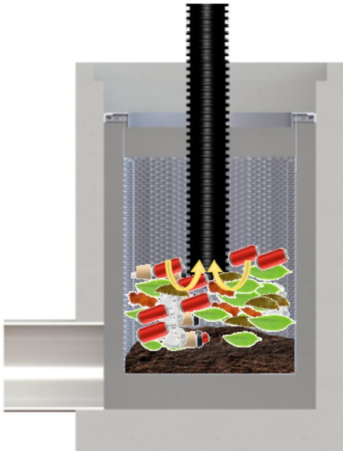
Insert the vacuum hose down into the filter basket and suck out debris. Use a pressure washer to assist in vacuum removal. Pressure wash off screens.
