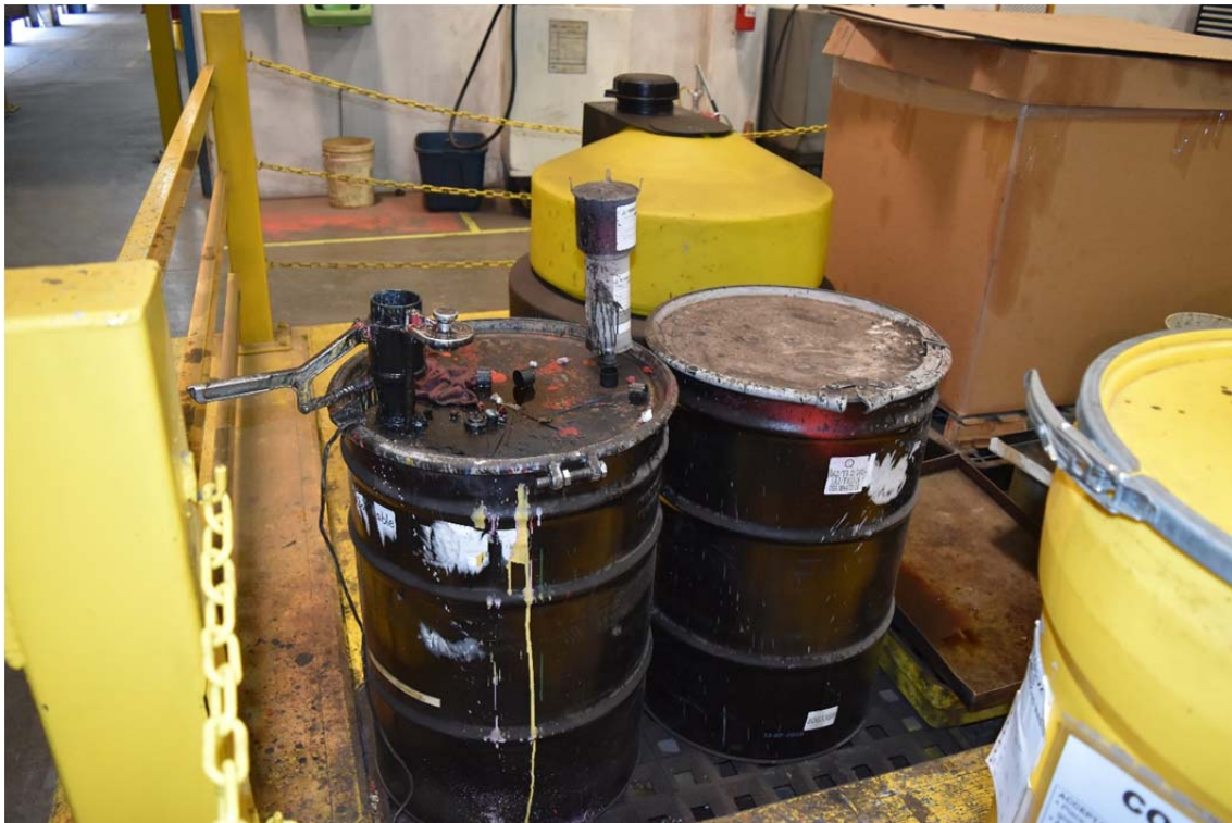
26. Waste oil storage drums within secondary containment in the maintenance area of the structure that are routinely removed under proper manifest.
