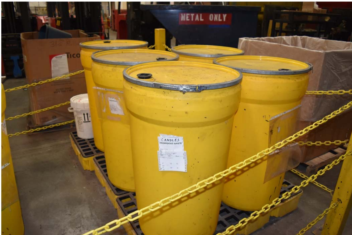
24. Waste storage area in the maintenance area in the southern portion of the structure on the central portion of the Site within secondary containment – wastes are routinely removed under proper manifest.
