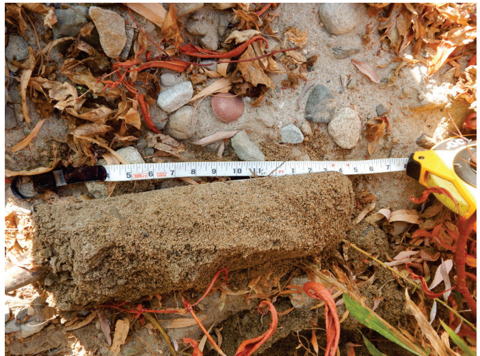
Sample Pit 1; soil type is coarse sand to cobble. The pit was dug in a problematic area. November 7, 2019.
