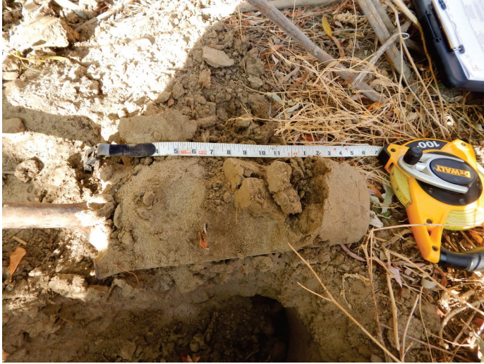
Sample Pit 2; soil type is sand to loamy fine sand, with sandy redox features present. November 7, 2019.
