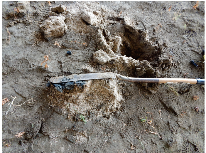
Sample Pit 10; soil type is coarse sand and clay. The pit was dug in a problematic area. November 7, 2019.
