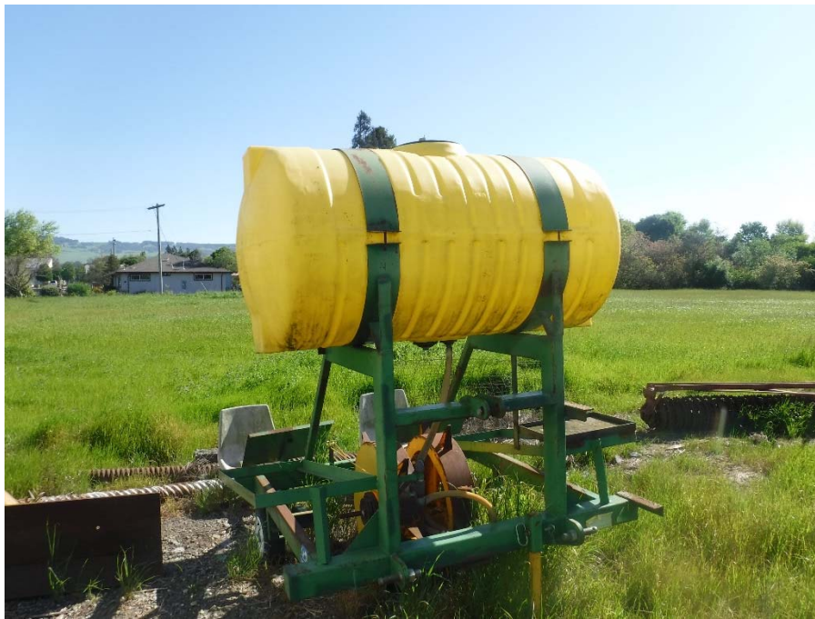
Photo 1: Above-ground storage tank mounted on trailer behind workshop. Empty, with some staining or residue on the bottom interior of the tank.
