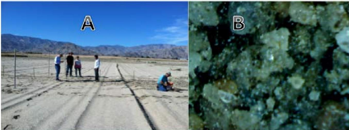
Figure 10: The CVARS solar-simulation site (A) and a hi-resolution in situ AMR image of the soil (3.01mm X 2.26mm, 100x image) showing soil particles.
