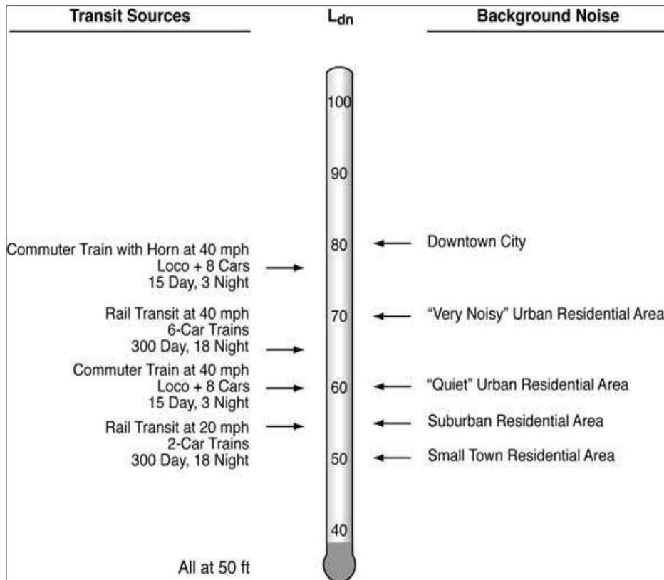
In addition to the Leq, Ldn, and SEL, another descriptor is used to describe noise. The loudest 1 second of noise over a measurement period, or Lmax, is used in many local and State ordinances for noise emitted from private land uses and for construction noise impact evaluations.
