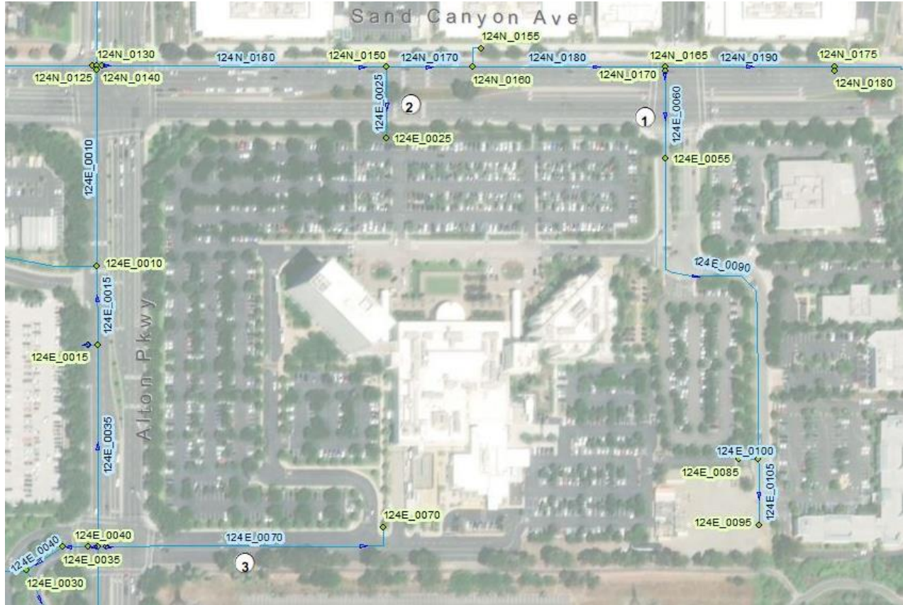
Figure 5. Recycled Water Model Pipe and Junction IDs
