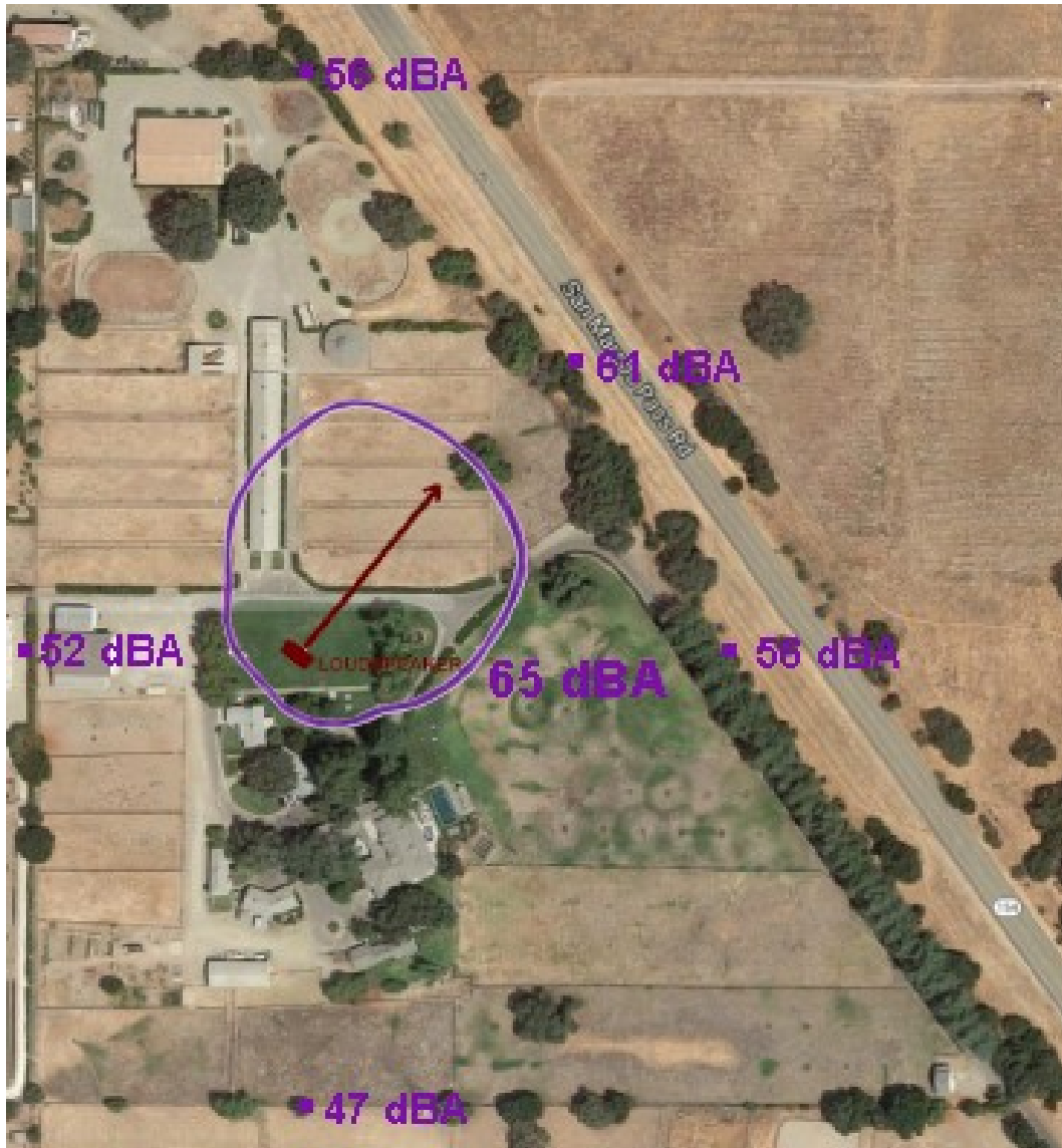
Figure 1: A-weighted Sound Levels from a Single Source Located at Position 1, north of the main house.
