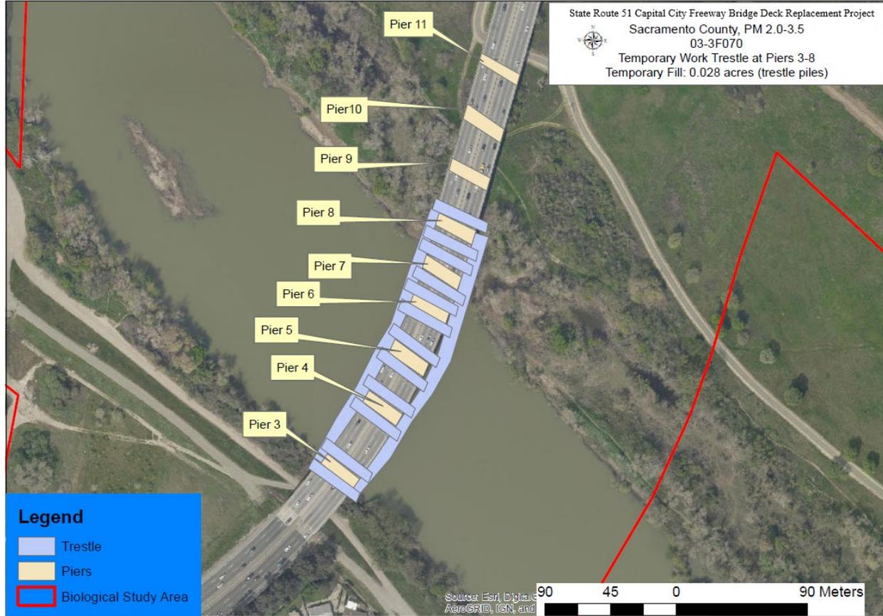
An impact hammer will drive the trestle piles. The trestle piles will likely require 400 blows/pile, totaling 800 blows per day (assuming two trestle piles driven per day). The final design for the temporary trestle will be determined by the contractor at the time of construction; the contractor may choose to use H-piles for the trestle instead of the steel pipe piles.
