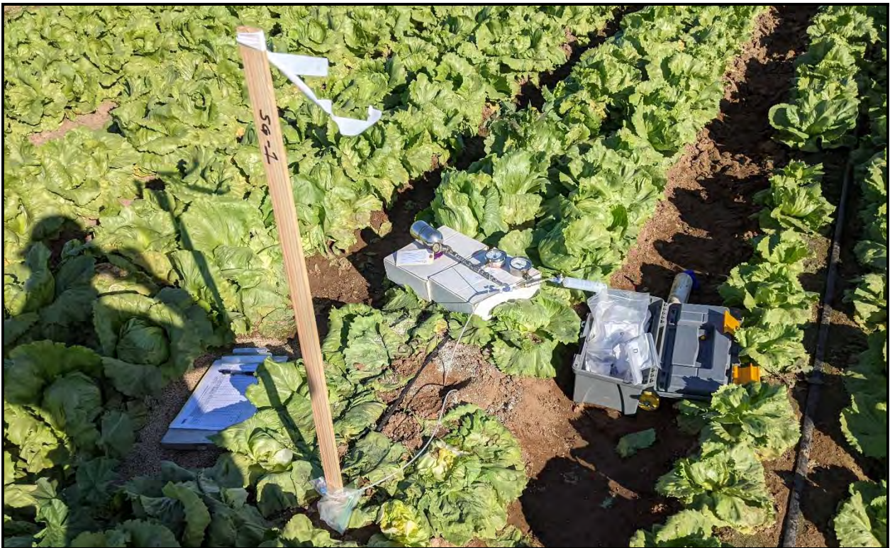
Photo 6. Soil gas location SG-1 during sample collection.
