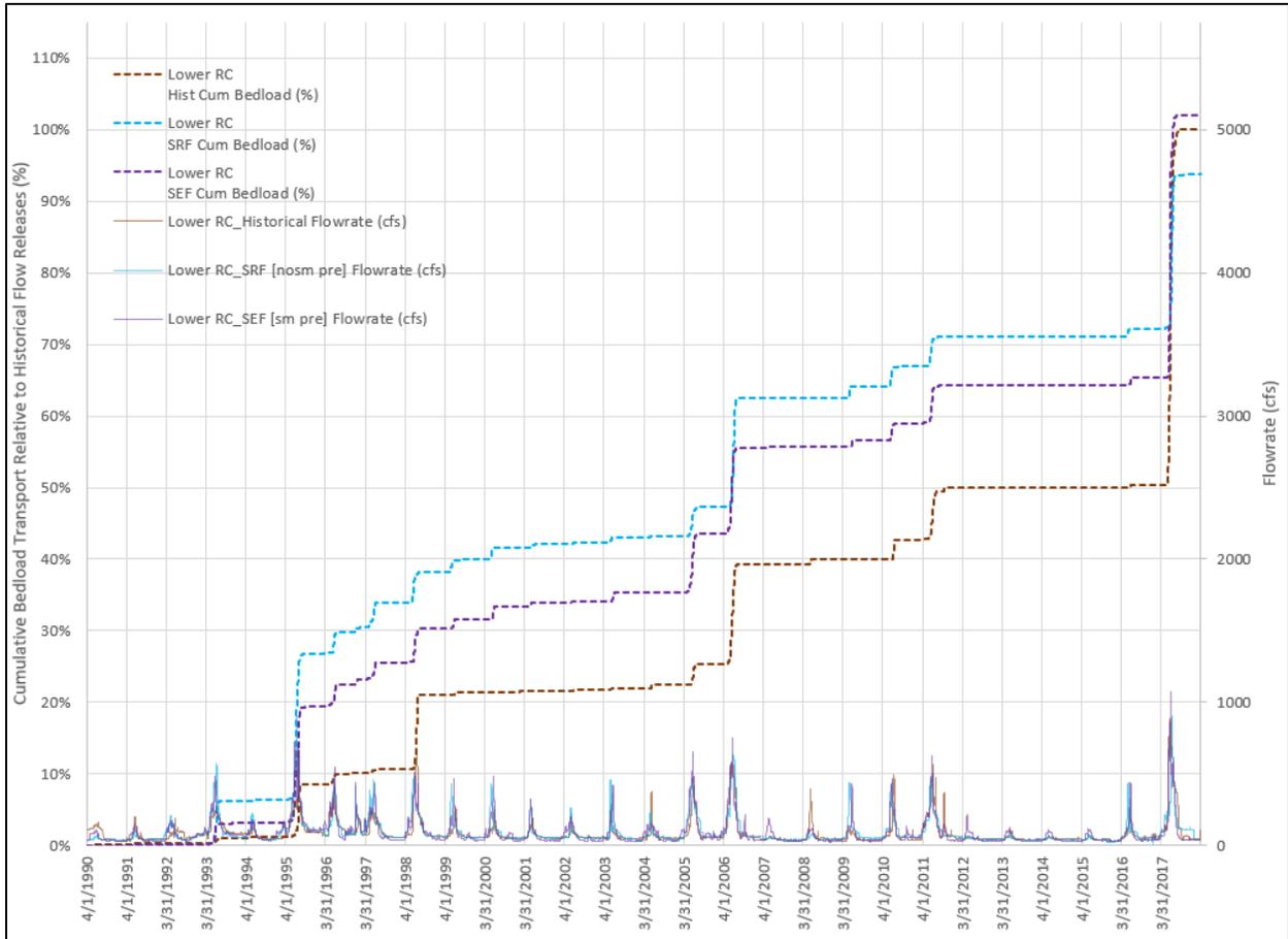
Figure 6. Lower Rush Creek, Below the Narrows, Cumulative Bedload Transport for Flow Regimes Relative to Historical Flow Releases using M&T Lower Rush Creek Bedload Site
