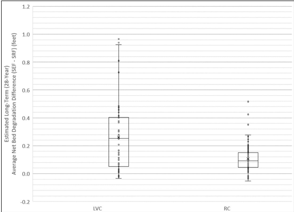
Figure 11. Box and Whisker Plots of Long-Term (28-Year) Average Net Bed Degradation Difference Results (SEF - SRF) by Creek
