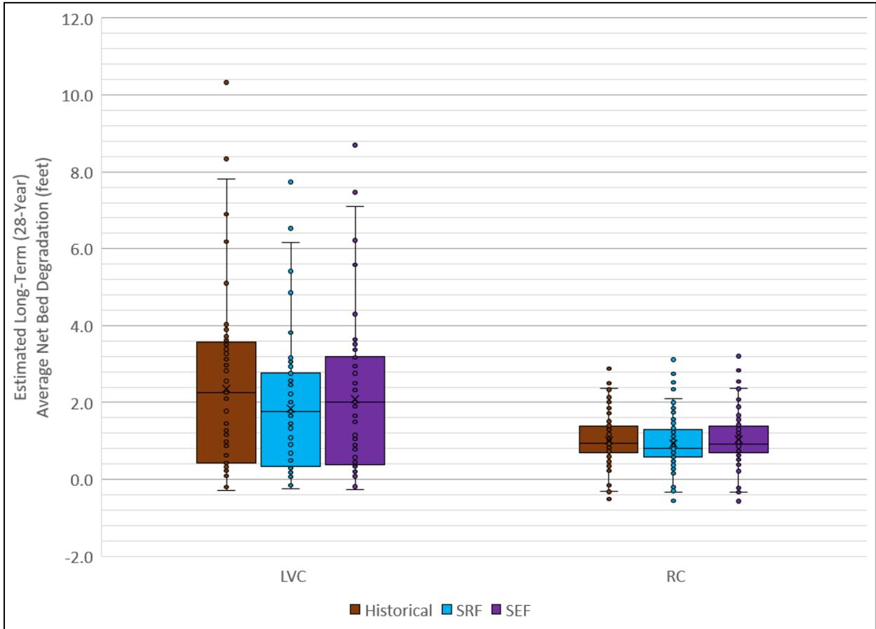
Figure 9. Box and Whisker Plots of Long-Term (28-Year) Average Net Bed Degradation Results by Creek
