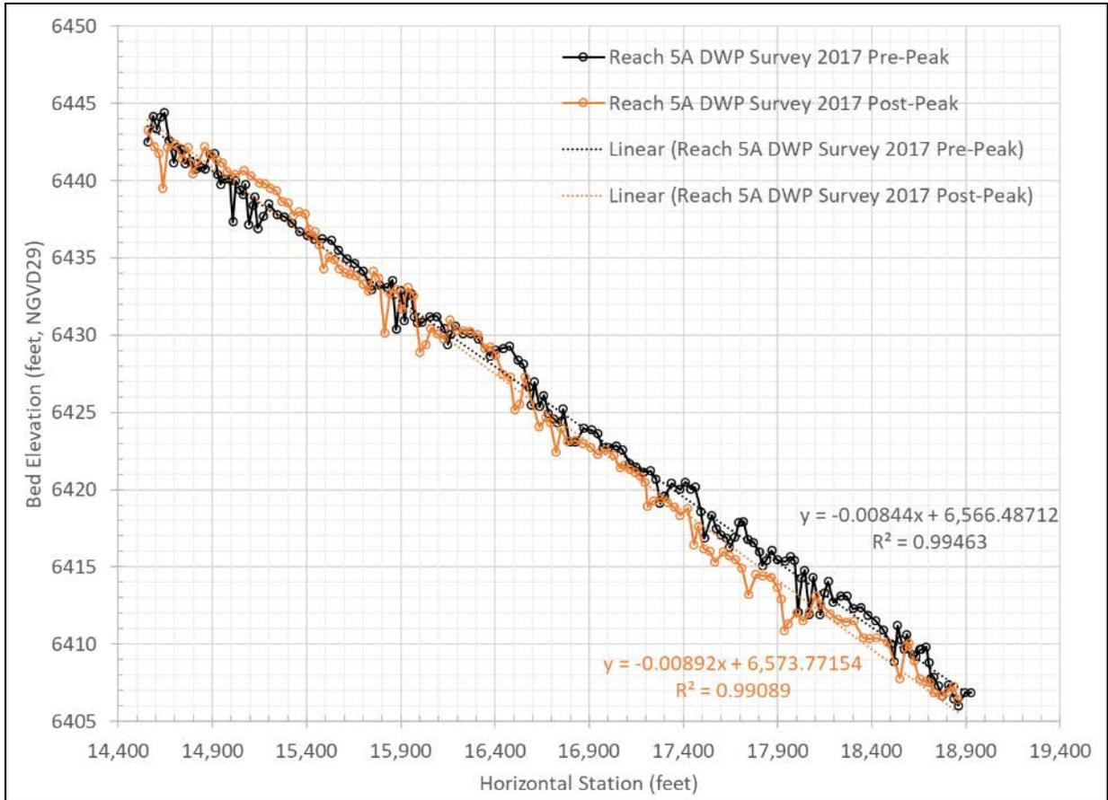
Figure 2. Example Historical Longitudinal Profile Survey Comparison – Rush Creek Reach 5A
