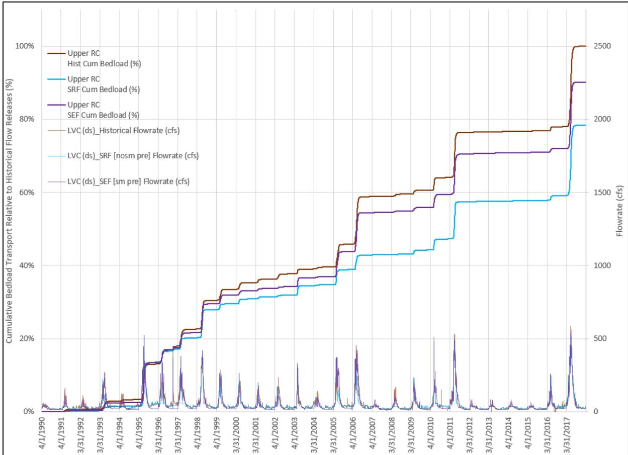
Figure 7. Lee Vining Creek, Below Intake, Cumulative Bedload Transport for Flow Regimes Relative to Historical Flow Releases using M&T Upper Rush Creek Bedload Site
