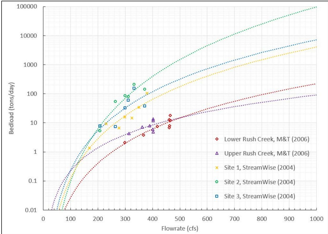
Figure 4. Bedload Data and Rating Curves
