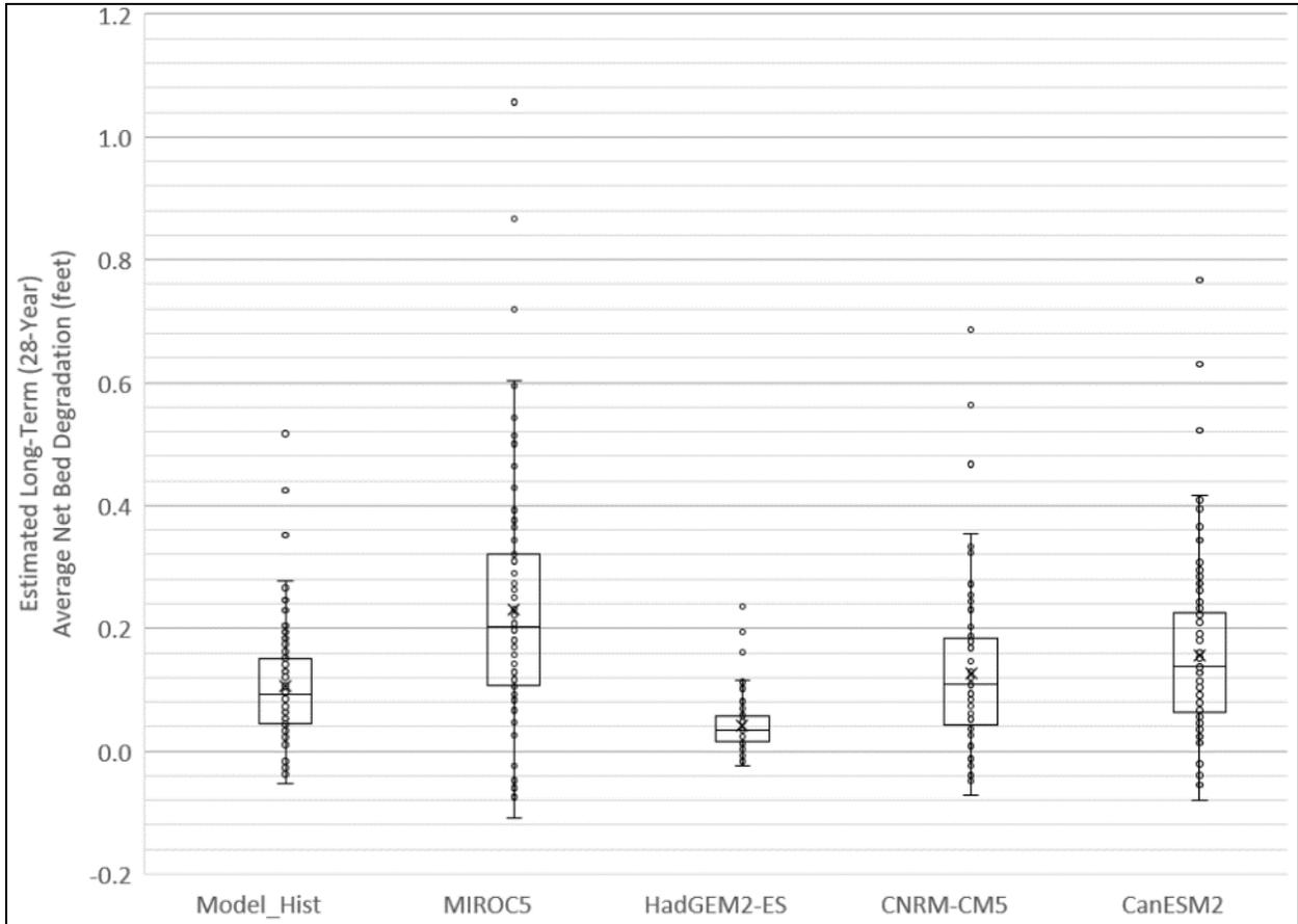
Figure 15. Box and Whisker Plots of Rush Creek Long-Term Bed Degradation Difference Results (SEF – SRF) for Climate Models
