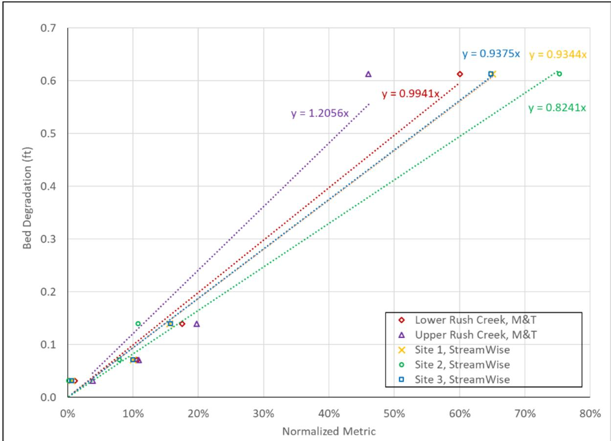
Figure 5. Example Relationship Between Normalized Bedload Transport and Bed Degradation – Rush Creek XS -09+82
