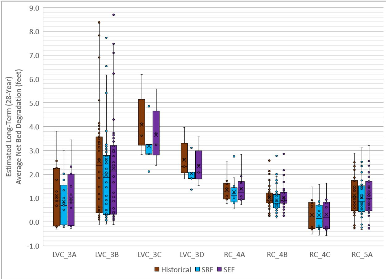
Figure 8. Box and Whisker Plots of Long-Term (28-Year) Average Net Bed Degradation Results by Reach
