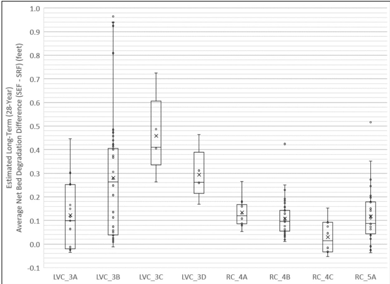
Figure 10. Box and Whisker Plots of Long-Term (28-Year) Average Net Bed Degradation Difference Results (SEF - SRF) by Reach
