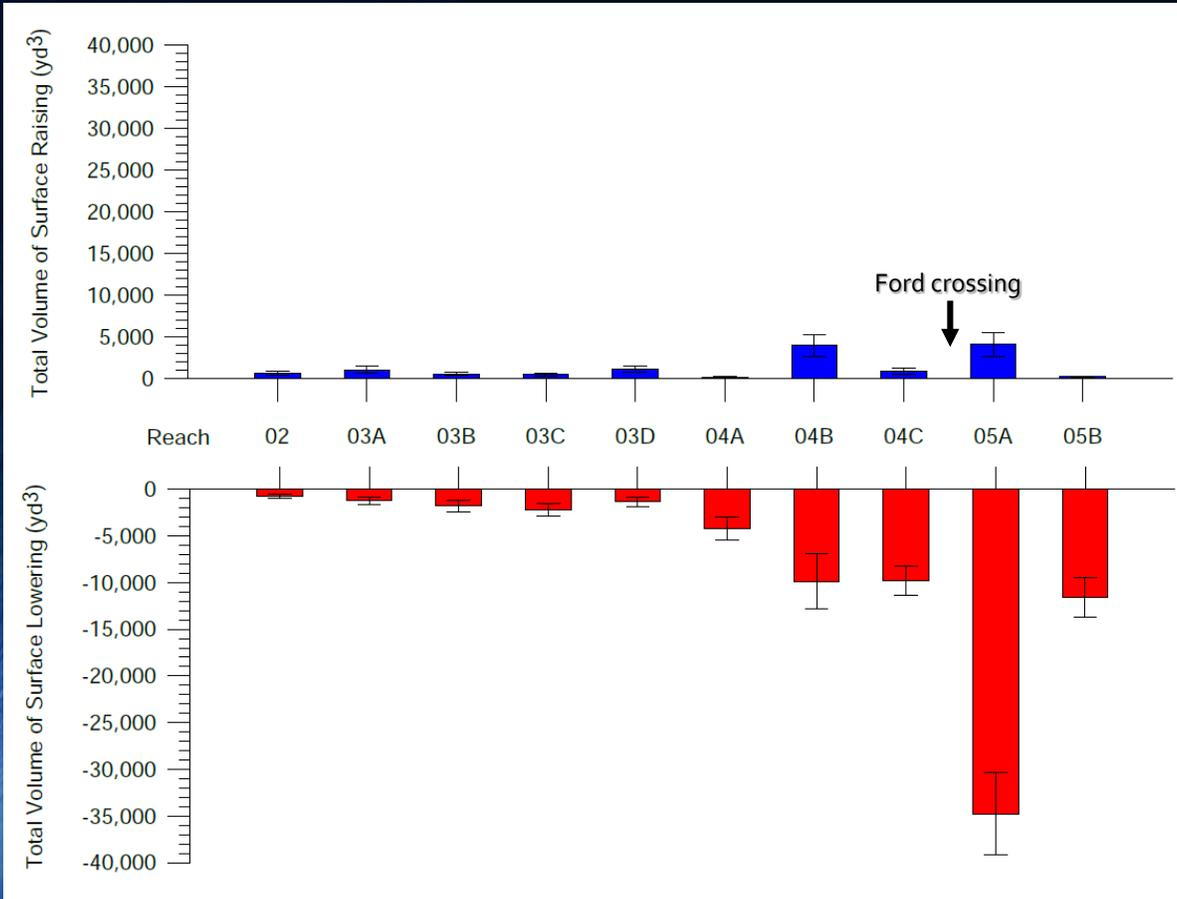
**Rush Creek:** Sediment transport imbalance illustrates that the vast majority of sediment moving through Upper and Lower Rush is exported to Mono Lake. Therefore, net channel lowering and riparian stranding is a primary consequence of increased peak flows associated with higher peak flows similar to the SEFs.
