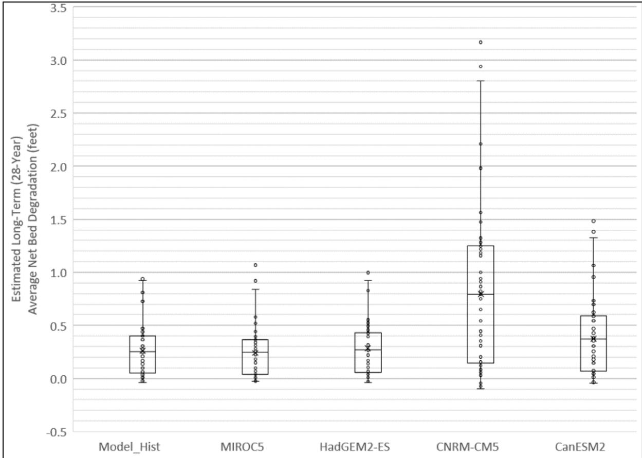
Figure 16. Box and Whisker Plots of Lee Vining Creek Long-Term Bed Degradation Difference Results (SEF – SRF) for Climate Models
