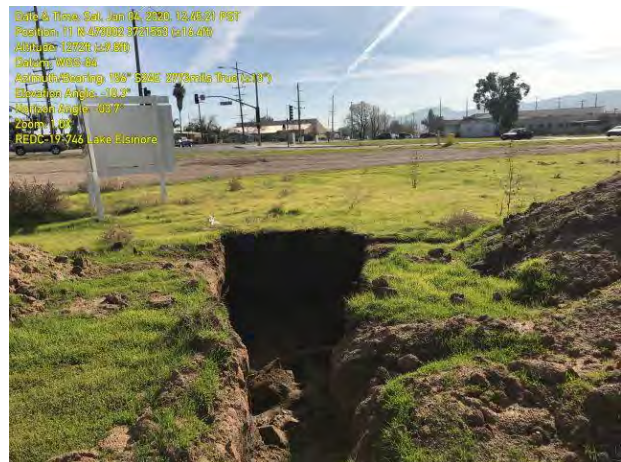
Photo 5. Soil test pit in the southeastern portion of the site, facing southeast (01.04.2020).
