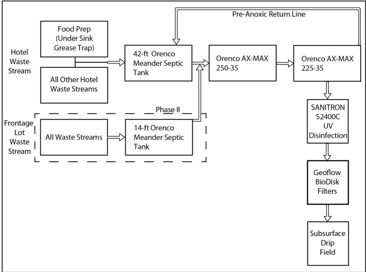
**Figure 2** Layout of the Wastewater Treatment System (Modified from Orenco Document NDA-ATX-1).
