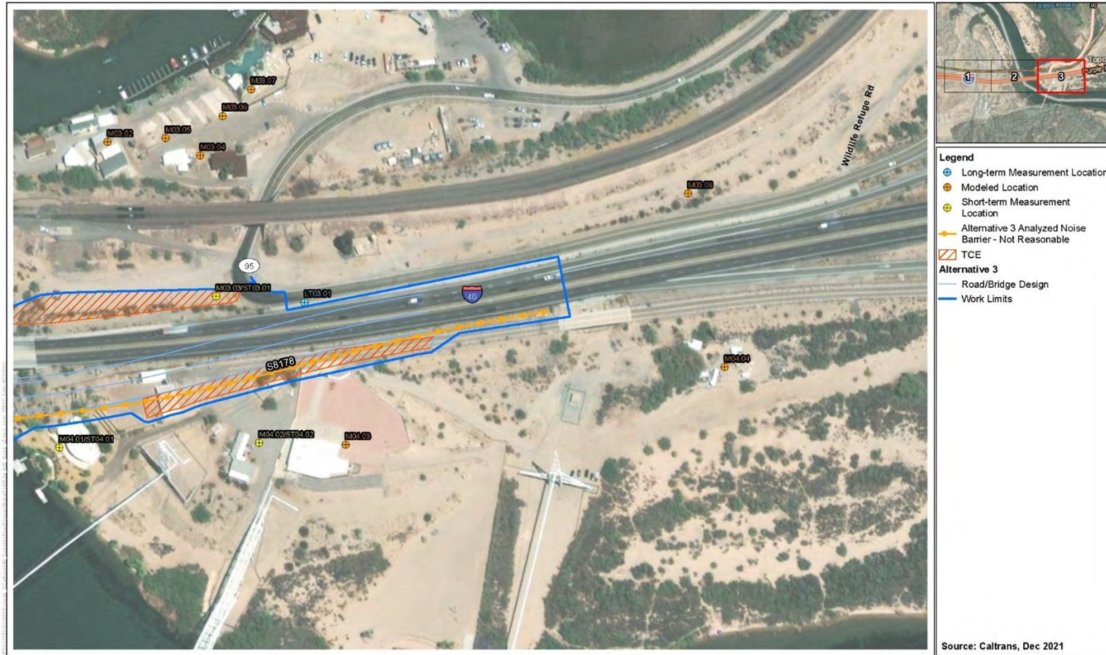
Alternative 3 Noise Measurement and Modeling Locations I-40 Colorado River Bridge Replacement Project
