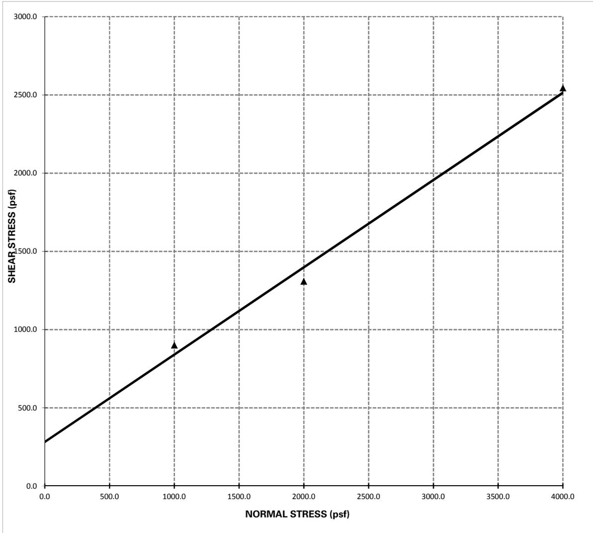
**Shear Strength:**  $\Phi = 29.2^\circ$  ; **C = 282.00 psf**
