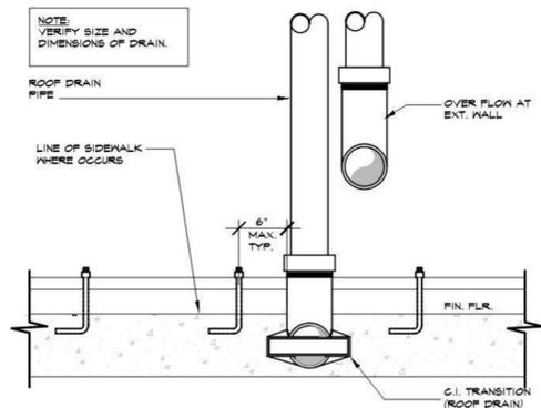
**ROOF DRAIN DISCHARGE THRU CONCRETE CURB**
