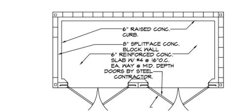
**TRASH ENCLOSURE FLOOR PLAN**
