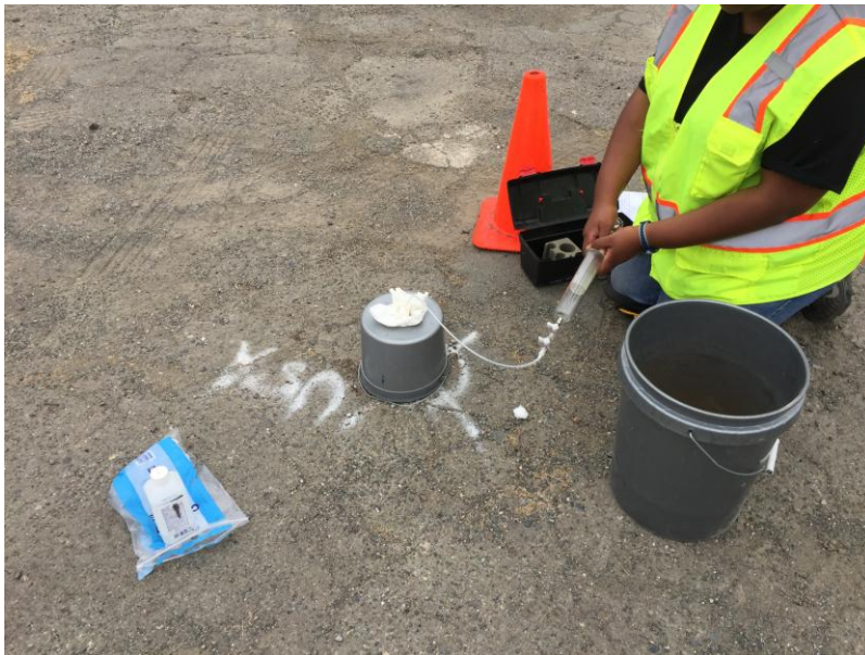
Photo 3: View collecting soil vapor sample in glass syringe, shroud and leak detection compound beneath connection
