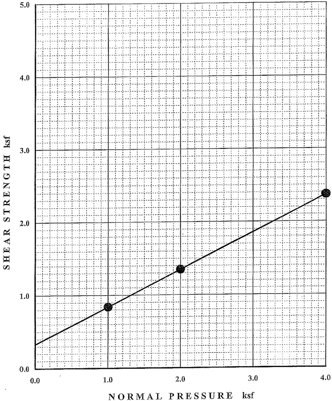
STRAIN RATE - 0.005 in/min      Initial moisture content = 24.6 %
