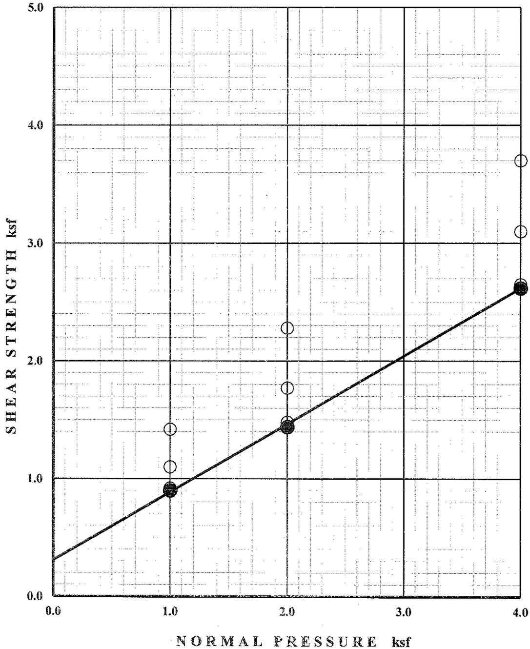
STRAIN RATE - 0.005 in/min Initial moisture content = 7.8 % Residual Re-Shear Resistance
