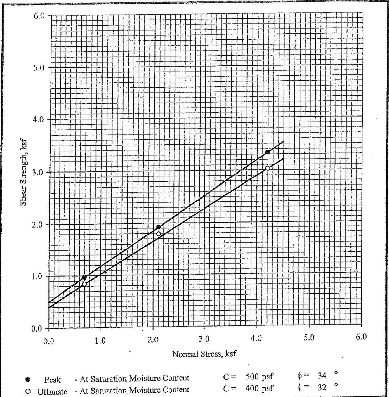
● Peak - At Saturation Moisture Content      C = 500 psf       $\phi = 34^\circ$
