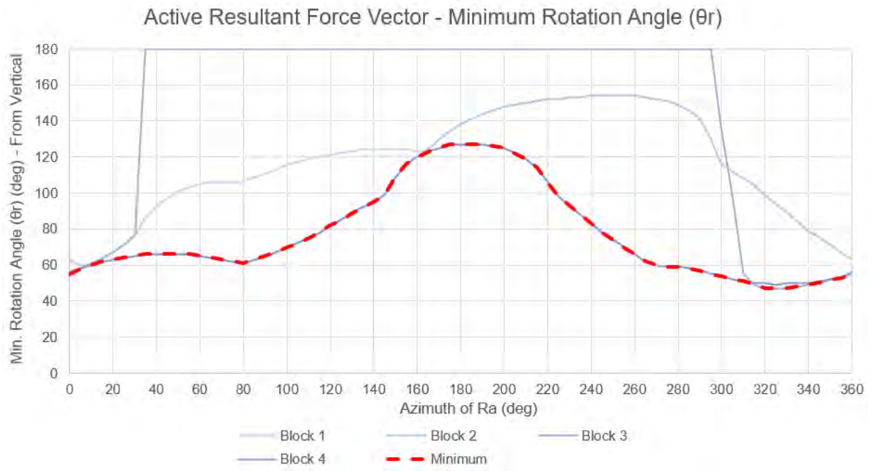
Figure 2-2. Determination of the minimum rotation angle of the active resultant force vector applied to removable block types from a flat (reference) slope.
