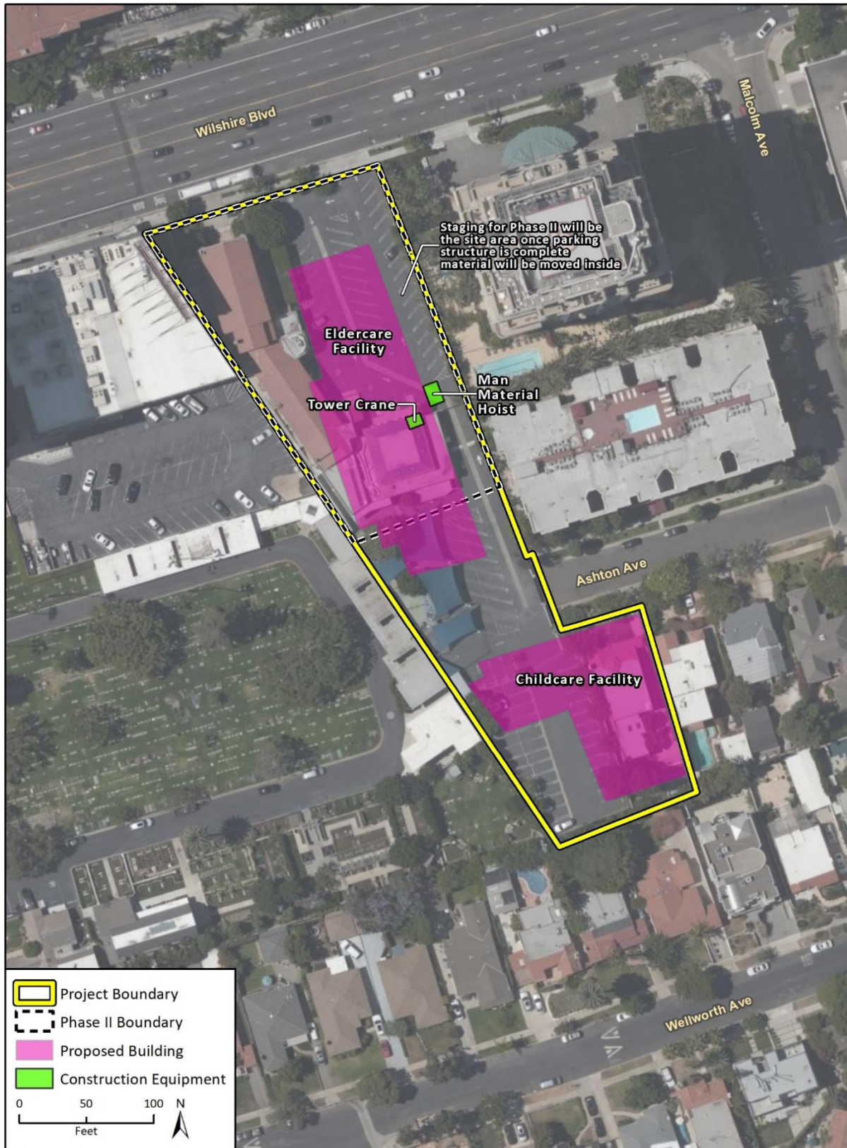
Figure 2-12 Phase II Staging
