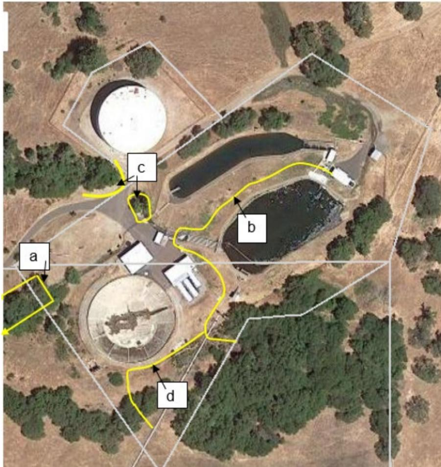
b = locate fencing at toe of fill
