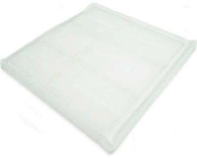
Paint Filter Pad, Polyester media with ECXL style. The media is multilayered, with finer fiber structures downstream in order to enhance depth loading capacity. The multiple layers will avoid face loading as it captures overspray paint with a downstream tackifier.
