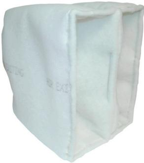
The recommended 2-stage system consists of a prefilter paint arrestor pad followed by a two pocket bag filter. This two pocket bag filter exceeds the approved EPA Method 319 testing requirements with or without the prefilter pad. The 2-pocket filter is self-sealing and has self supporting pockets. The Media construction is a multi-layered gradient density structure to maximize paint collection and retention.
