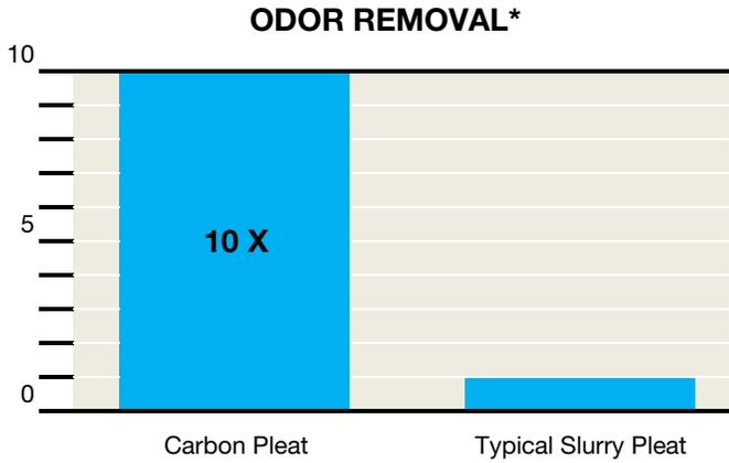
\*Amount of gas or odor removed at 50% break through given 880 PPM of Toluene @ 40 (media velocity)
