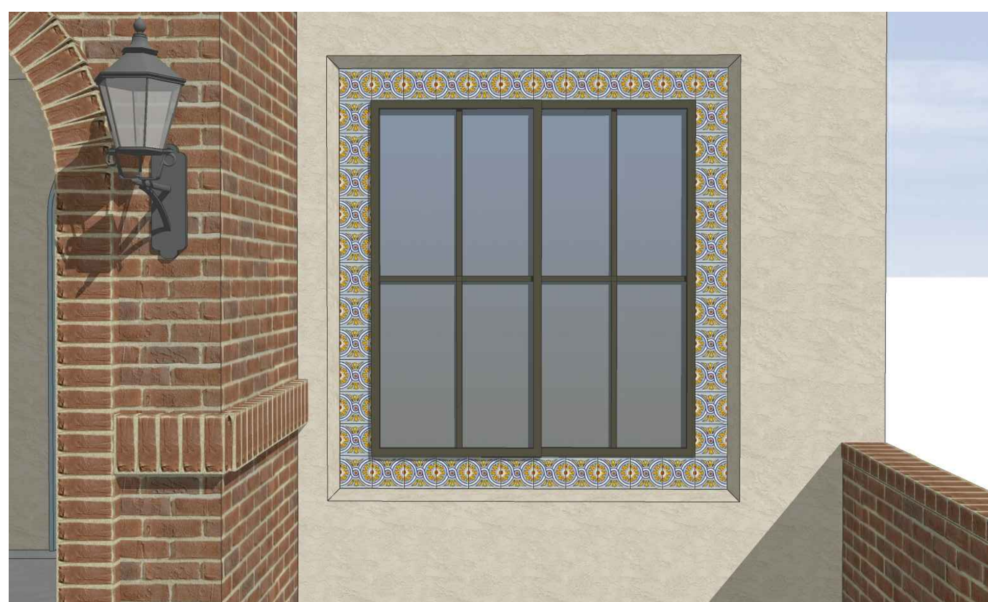
Tile Window Surround
