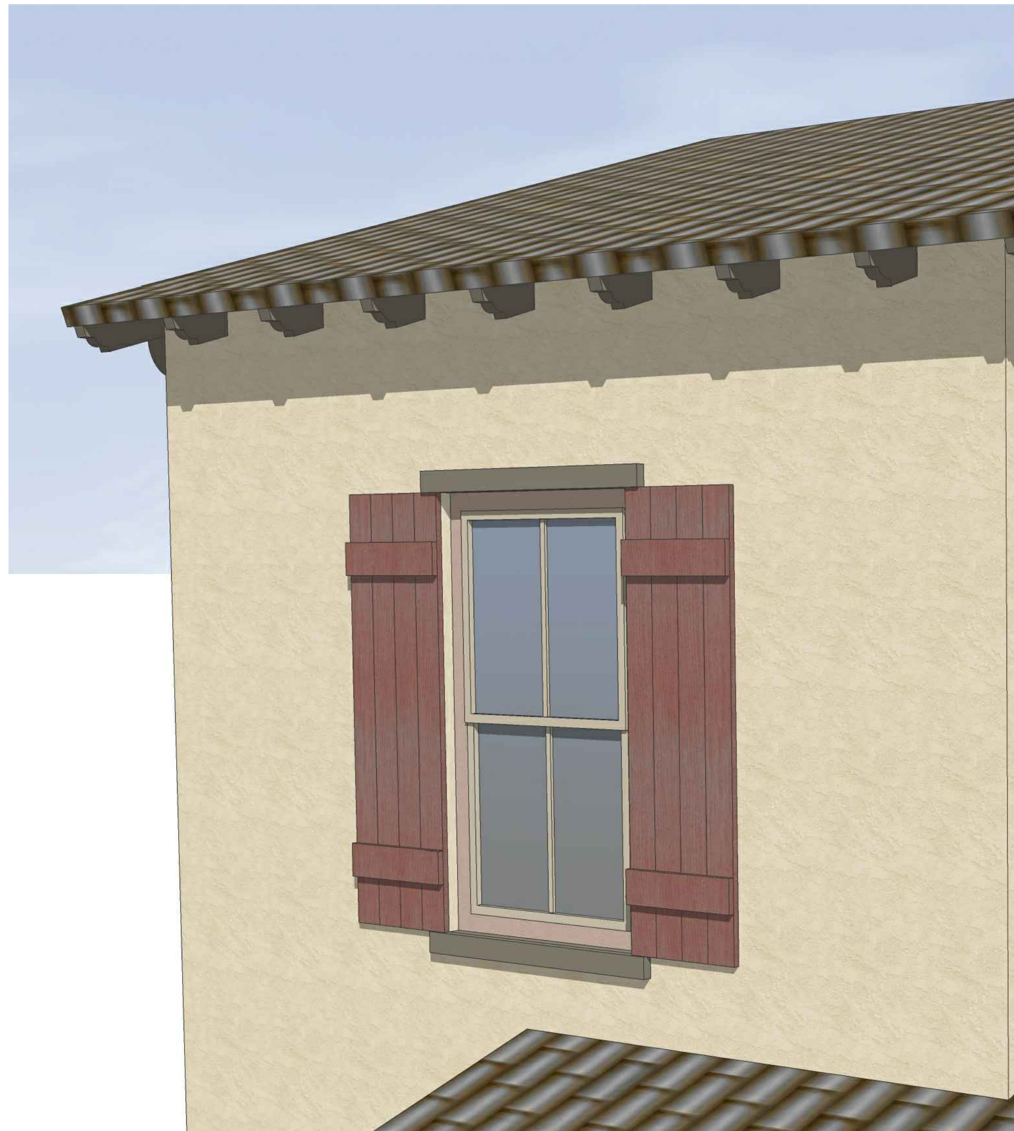
Recessed Window with Shutters
