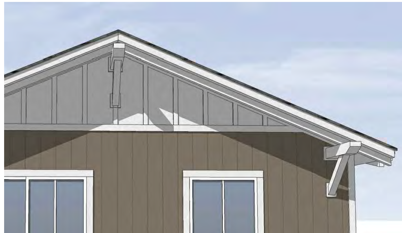
Gable End Detail with Siding
