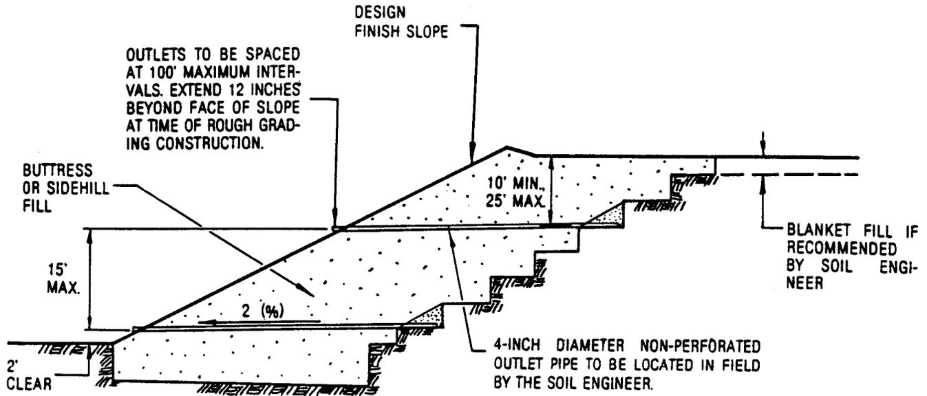
FILTER MATERIAL TO MEET FOLLOWING SPECIFICATION OR APPROVED EQUIVALENT: (CONFORMS TO MA STD. PLAN 323)
