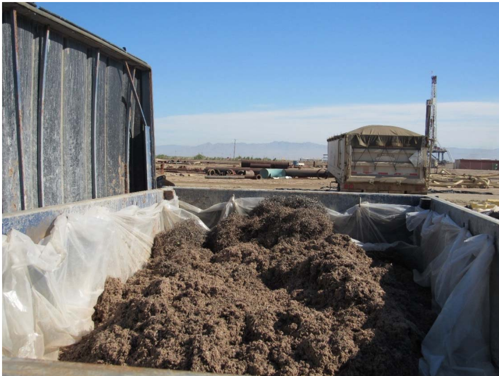
Photo 34: Looking at container with drilling mud with metal shavings located within the storage area of the Plant Site.
