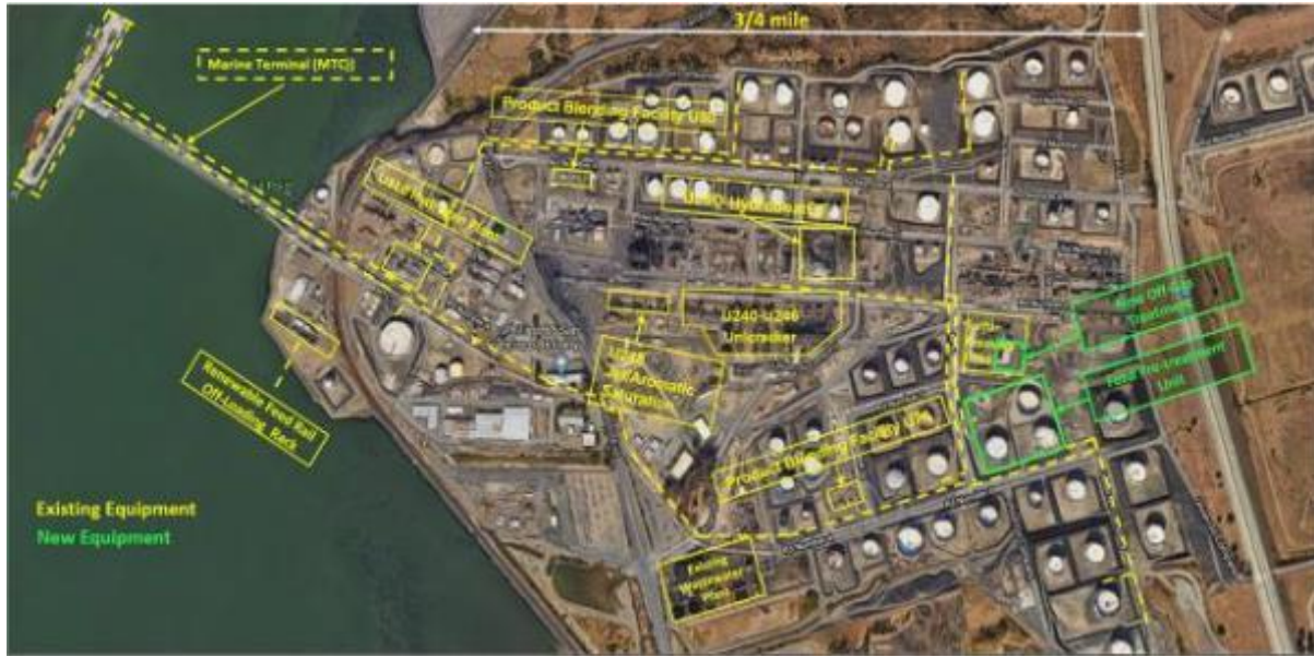
Figure 4.2-12 Rodeo Site Location of Existing Equipment and Proposed New Equipment
