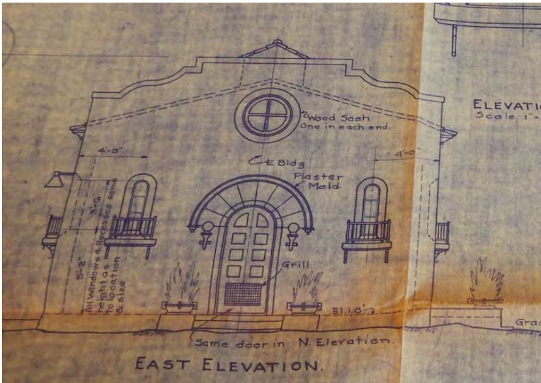
Figure 14. Excerpt from 1926 as-builts depicting the eastern (primary) elevation of the former substation at 498 Del Monte Avenue. The rose window has been infilled, and the sconces flanking the door have been removed. Based on inspection of an aerial from 1929 (Figure 15), the decorative planters on either side of the doorway in the as-builts never were installed.
