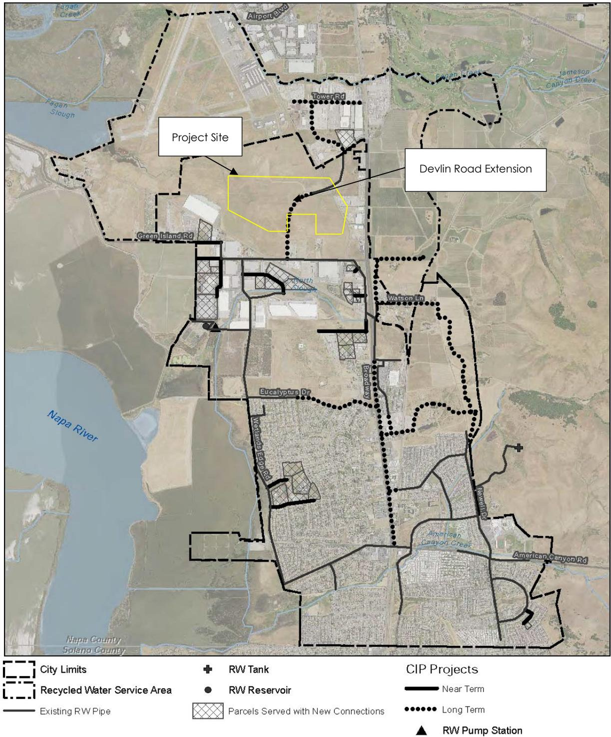
**Figure 1-3 Existing and Planned Recycled Water System for the City of American Canyon, California.** As reported in the City of American Canyon Recycled Water Master Plan, 2016.
