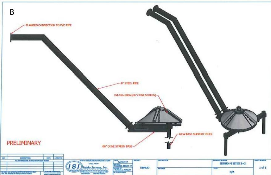
Figure 5. Schematics of existing water diversions with the addition of proposed 66 inch (approximate) cone fish screen with self-cleaning brush system at A) Site 1 and B) Site 2 and Site 3 in the lower Mokelumne River.
