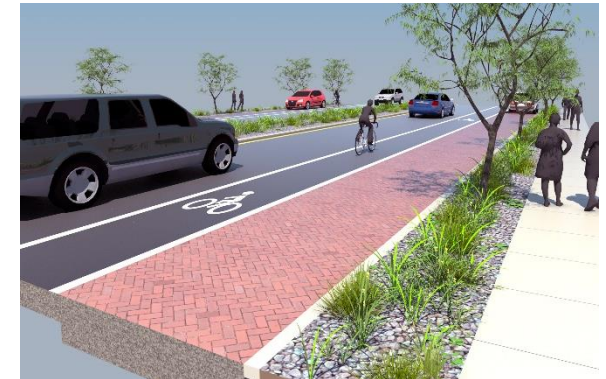
Green street with permeable pavement in parking lane
