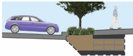
STRUCTURAL CELLS Manufactured cells support the sidewalk allowing uncompacted soil to promote tree roots to grow below.
