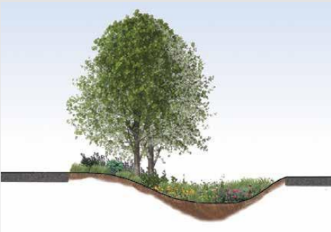
Water is infiltrated into the ground, evapotranspired by plants or drained
