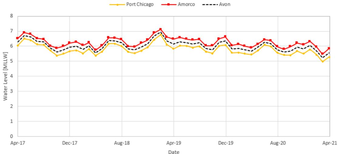
**Figure 6 – Highest Observed Water Levels from April 2017 to April 2021.**
