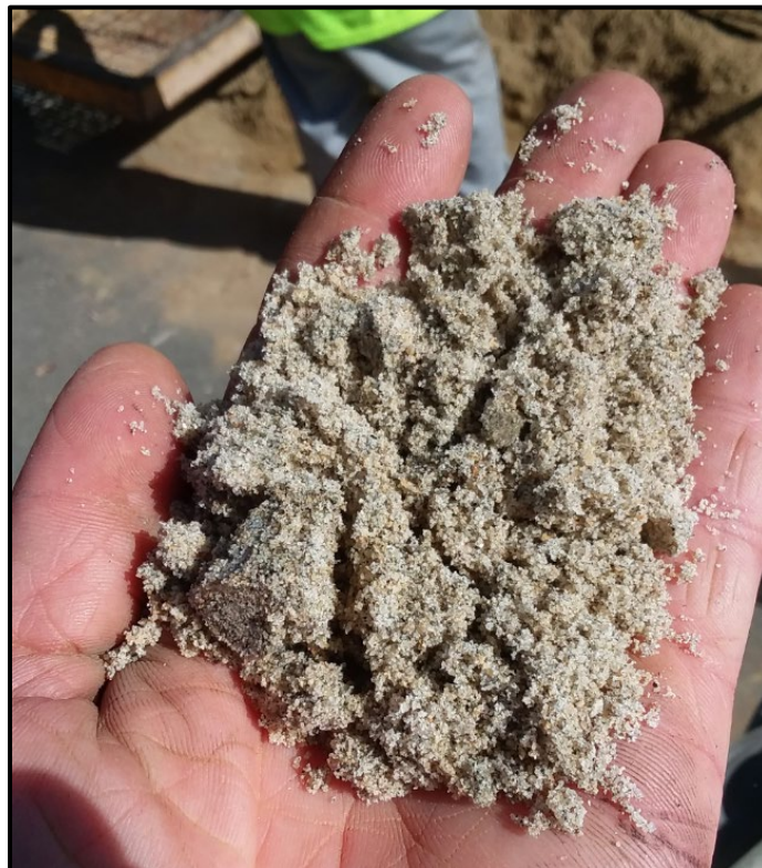
Figure 4-4. Unit 2 Paralic Deposits (Poorly-Graded Sands) at Depth
