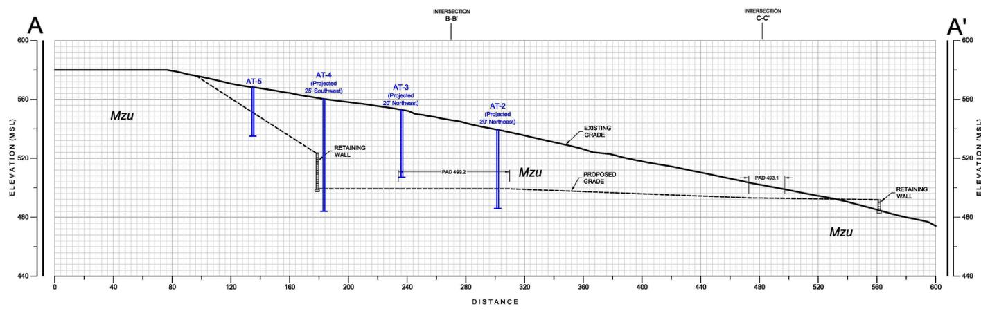
**GEOLOGIC CROSS-SECTION A-A'**
