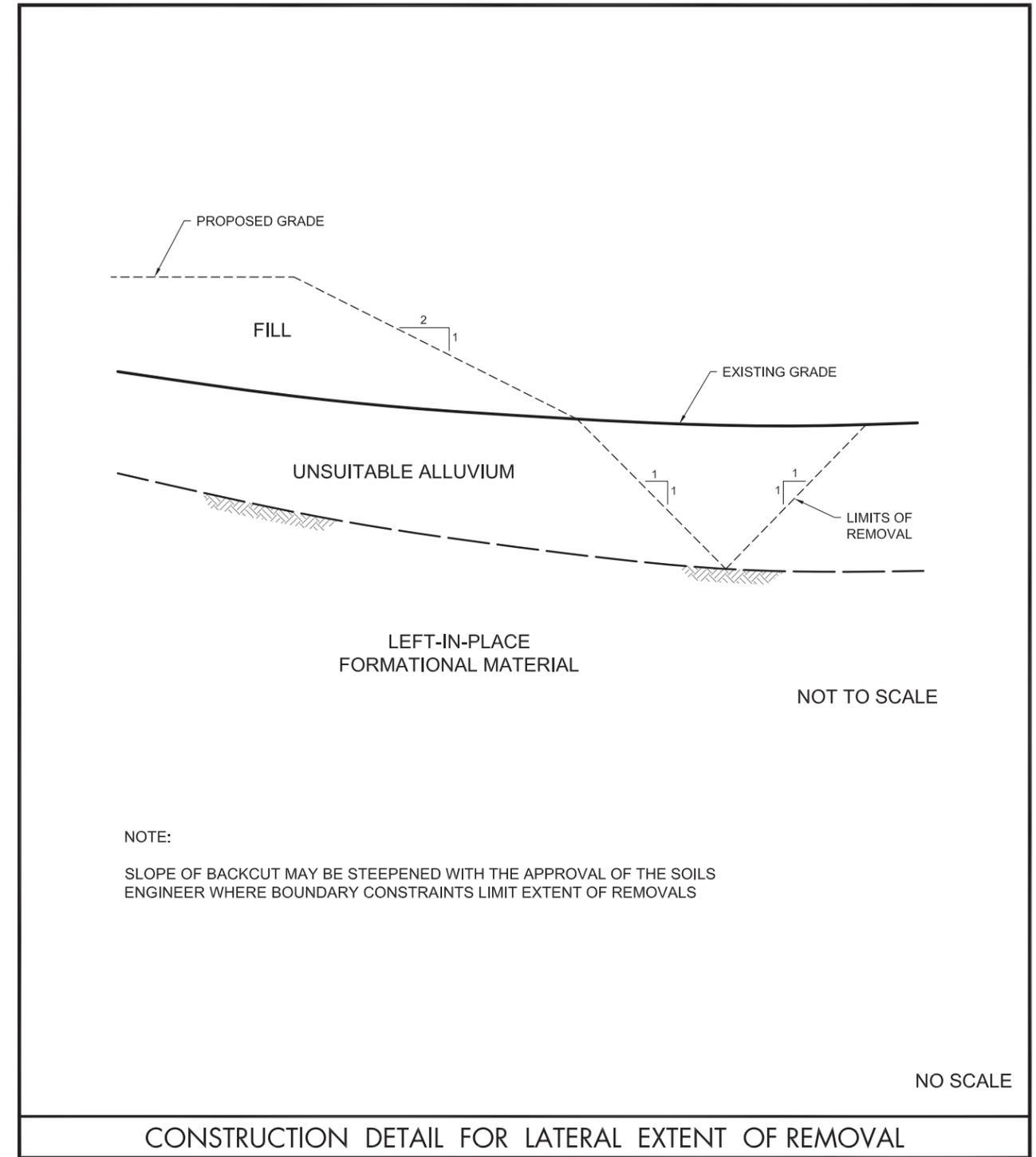
CONSTRUCTION DETAIL FOR LATERAL EXTENT OF REMOVAL
