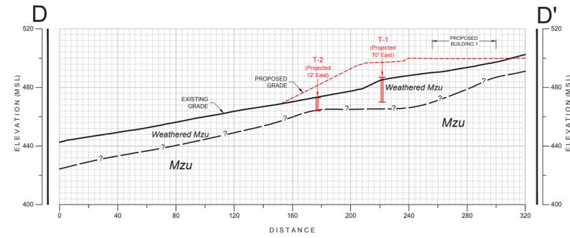
**GEOLOGIC CROSS-SECTION D-D'**
