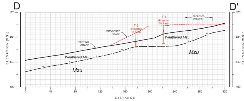
**GEOLOGIC CROSS-SECTION D-D'**
