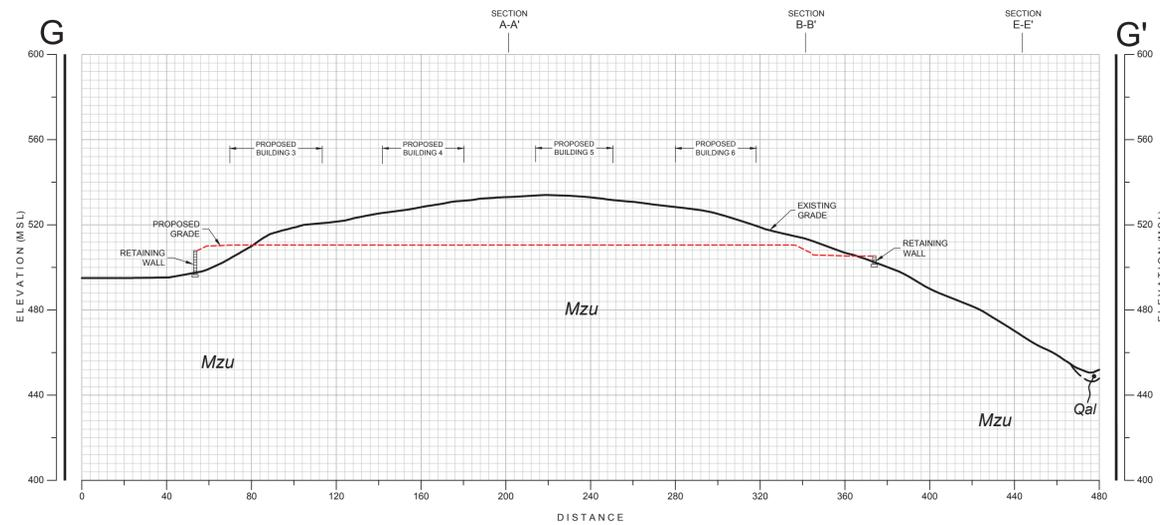
**GEOLOGIC CROSS-SECTION G-G'**
