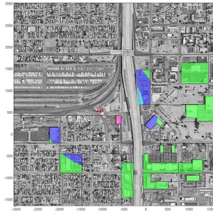
Upper Bound Damage at Pre-Engineered Bldgs (Explosion)
