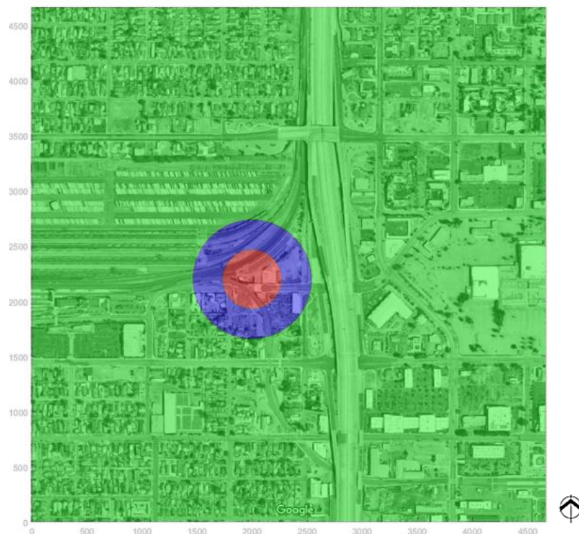
Figure 12 – Expected Extents of Cracked Glass (blue) and Structural Damage (red) for GH2 (265-kg) Scenarios
