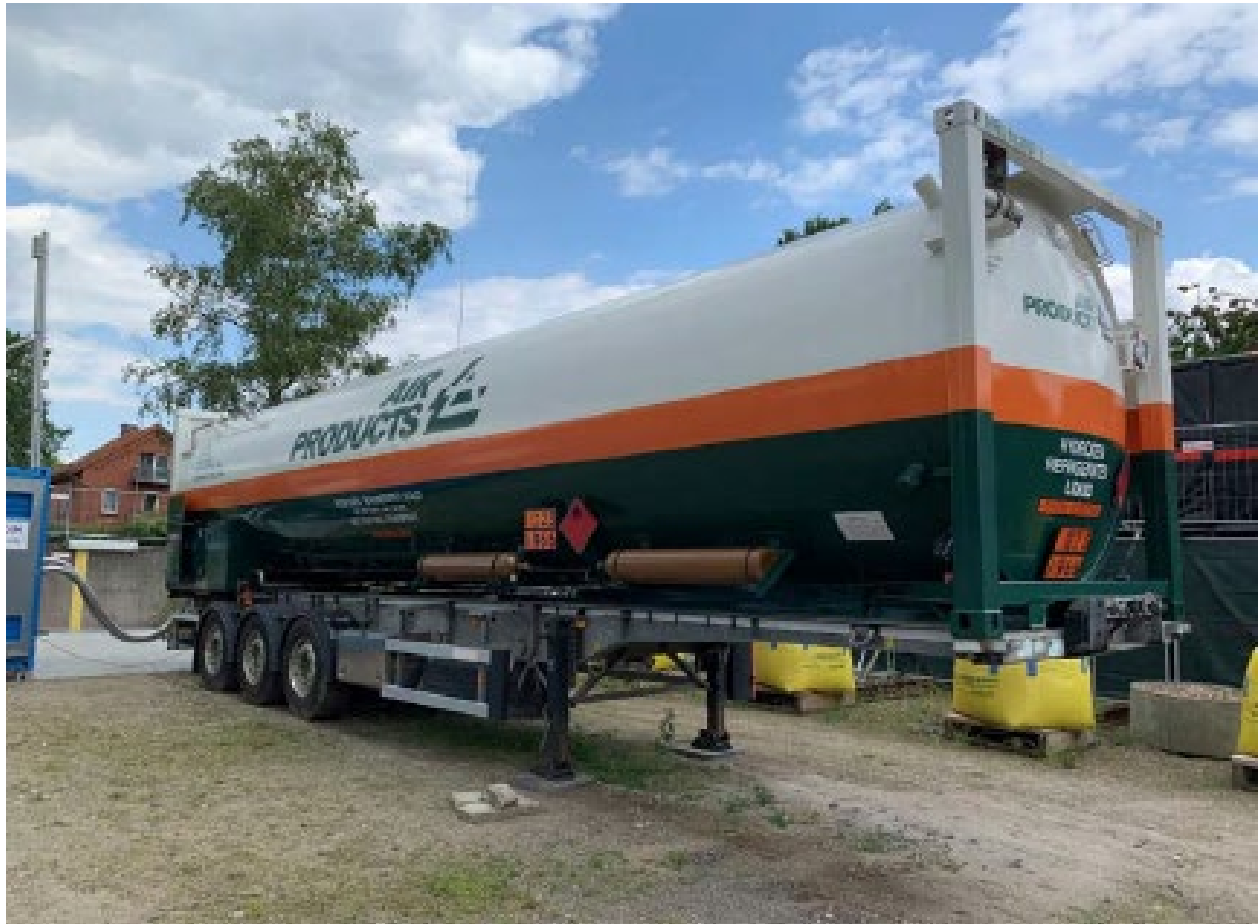
Figure 2-4. Example Hydrogen Fuel Storage Tank
