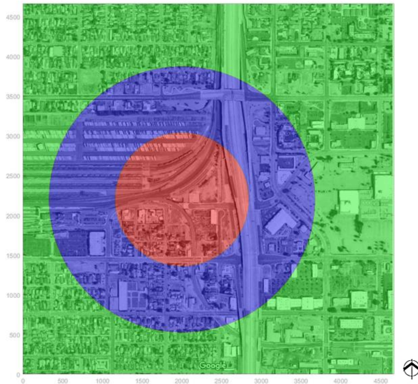
Figure 13 – Expected Extents of Cracked Glass (blue) and Structural Damage (red) for LH2 (4000-kg) Scenarios
