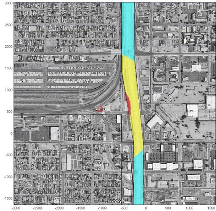
Upper Bound Damage at Elevated Roadways (Explosion)
