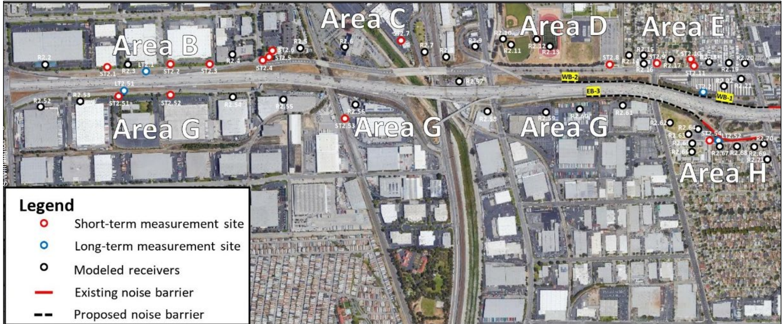
Figure 2.13-3. Analysis Areas, Noise Monitoring Positions, and Location of Evaluated Noise Barrier (Eastern Most Terminus)
