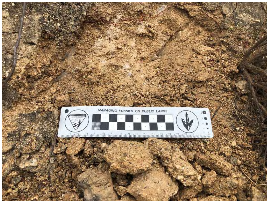
Figure 6. Strata of the “sandstone of Wildomar area” as exposed in the steep slope along the northwestern border of the Project site, consisting of tan, massive, poorly consolidated, coarse- to very coarse-grained gritty sandstone.
