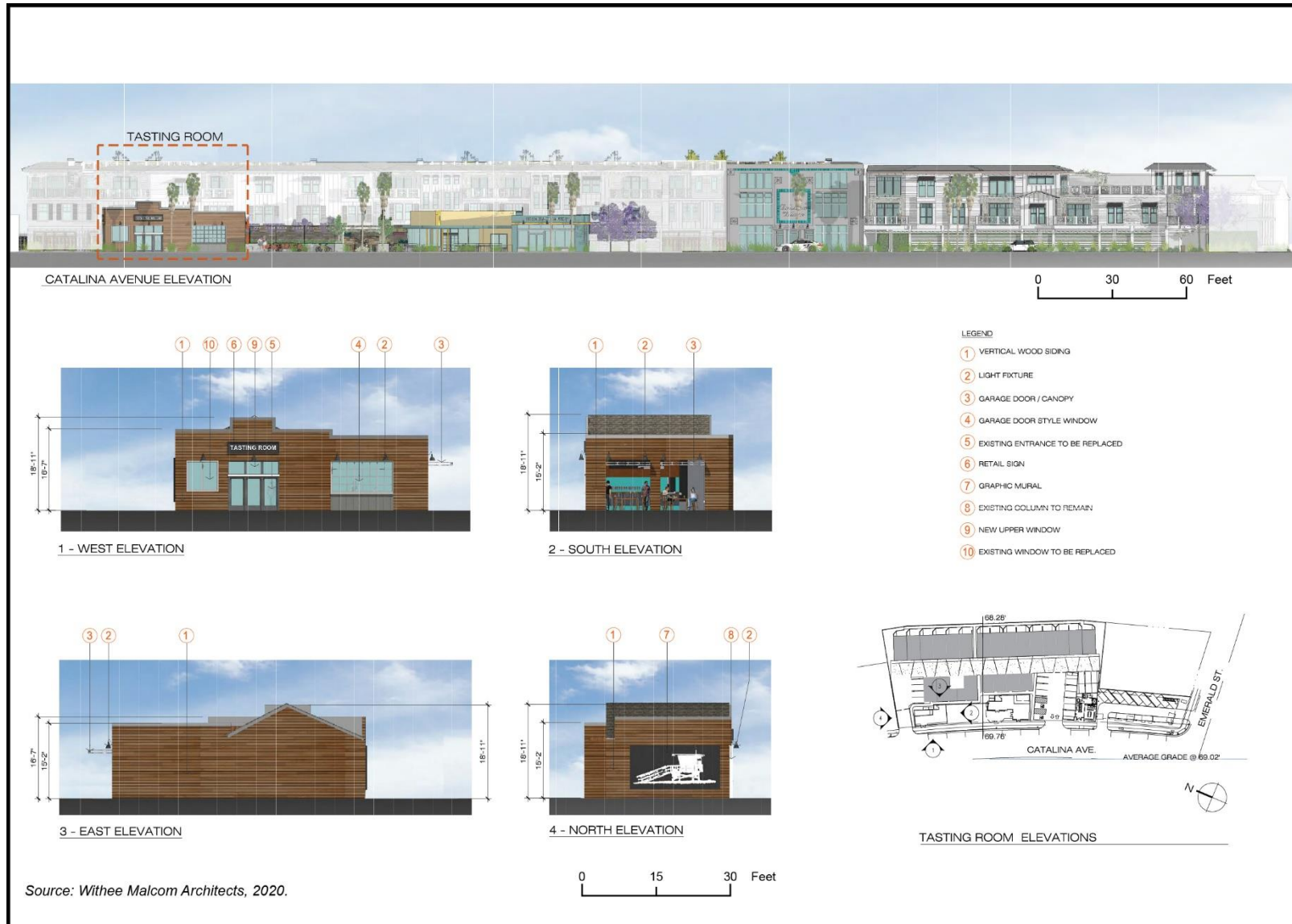
Figure 8 Project Elevations – Tasting Room
