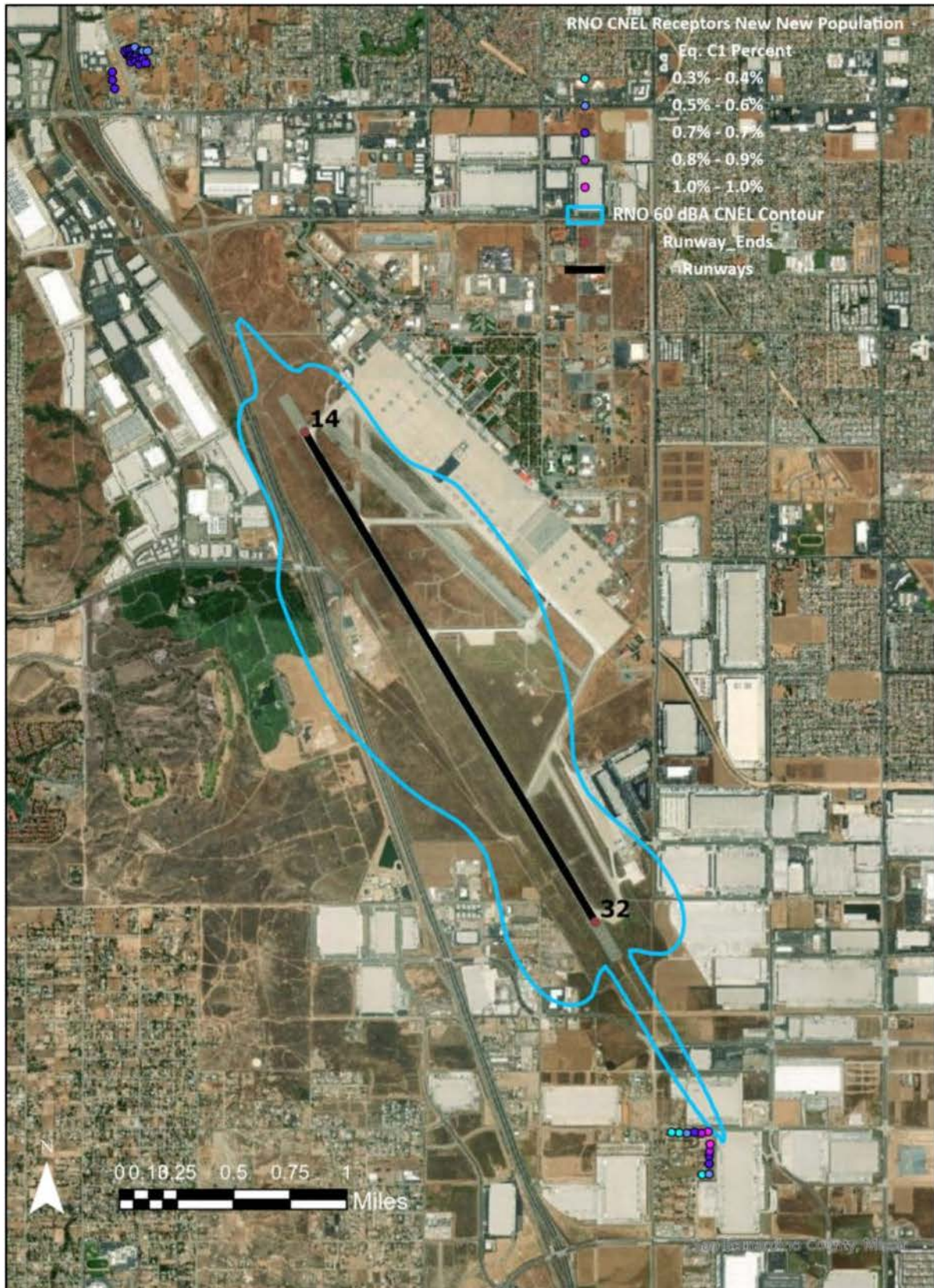
Figure 8C: Reduced Night Operations CNEL Contour and Percent of New Population Potentially Awakened
