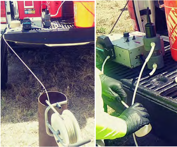
On base monitoring well being sampled for PFAS
