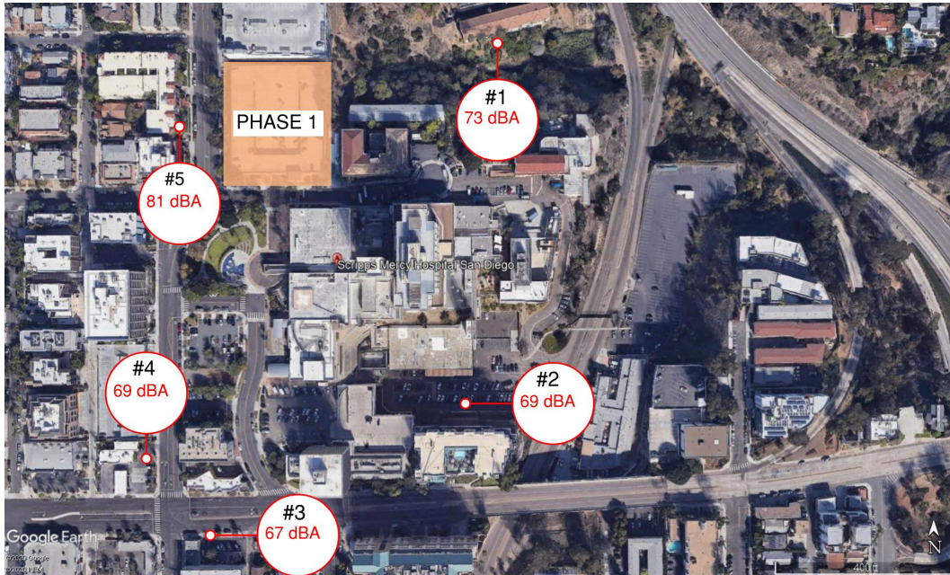
Figure 7 - Parking Lot 4.1 Demolition phase - total sound levels during allowed construction hours, at five receiver locations for the demolition period
