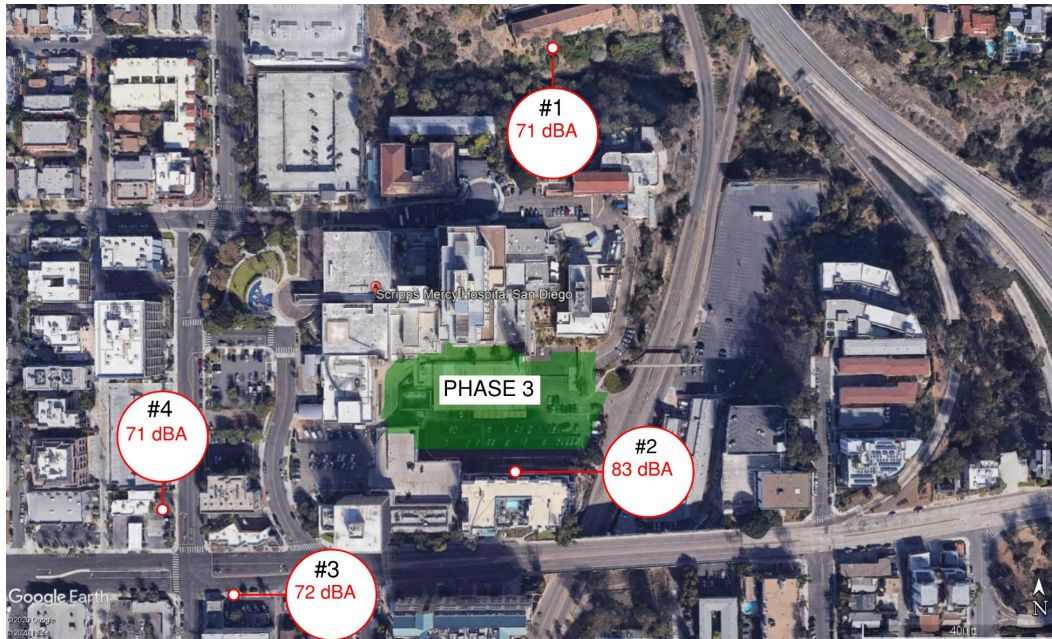
Figure 9 – Behavioral Health Building Demolition phase - total sound levels during allowed construction hours, at four receiver locations for the demolition period
