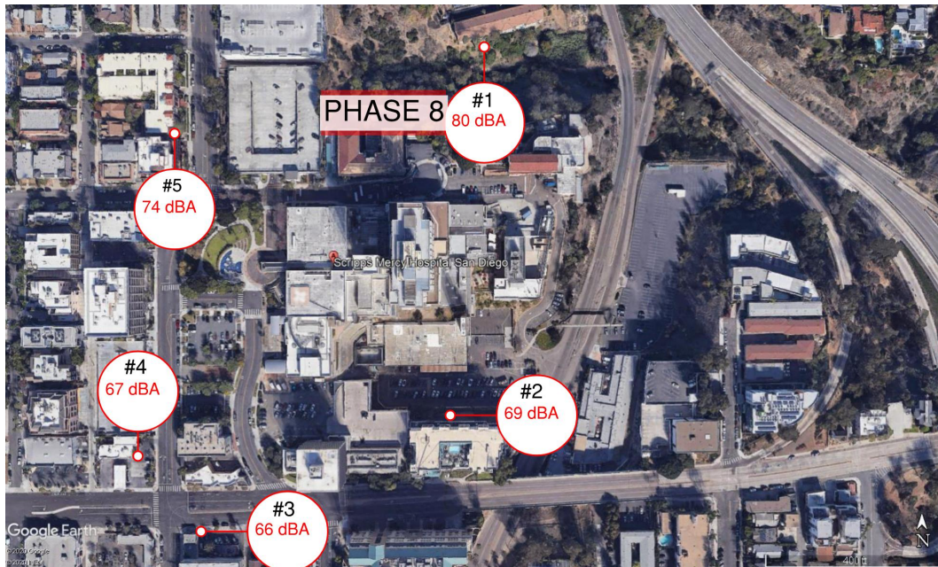
Figure 14 – Mercy Manor Demolition phase - total sound levels during allowed construction hours, at five receiver locations for the demolition period
