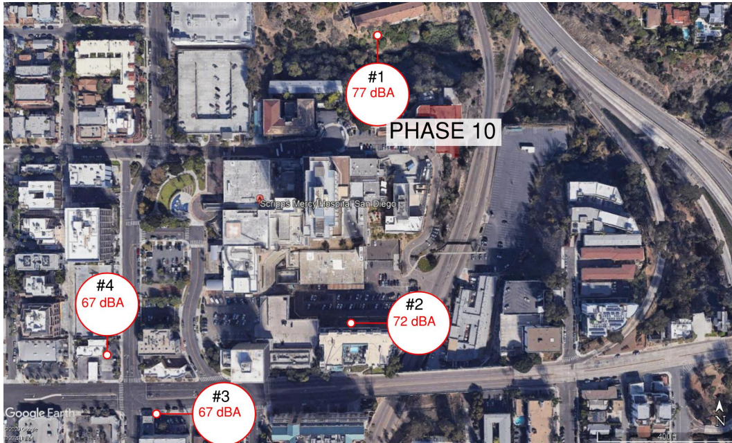
Figure 16 - Facility and Generator Building Demolition phase - total sound levels during allowed construction hours, at four receiver locations for the demolition period
