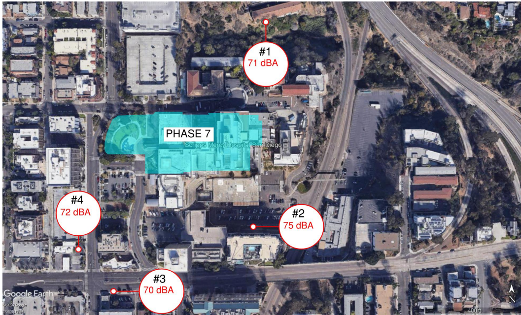
Figure 13 - Existing Hospital Demolition phase - total sound levels during allowed construction hours, at four receiver locations for the demolition period
