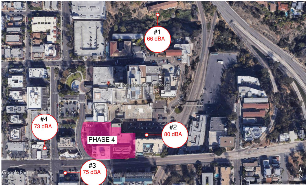
Figure 10 - 550 Washington Demolition phase - total sound levels during allowed construction hours, at four receiver locations for the demolition period
