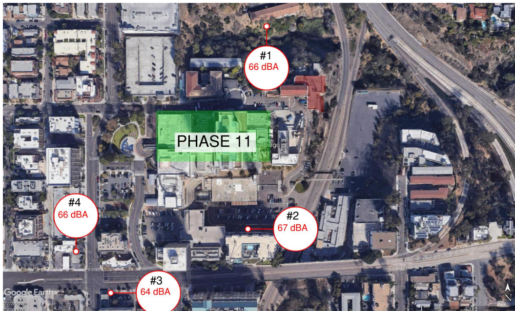
Figure 17 - Hospital II Construction - total sound levels during allowed construction hours, at four receiver locations for the demolition period
