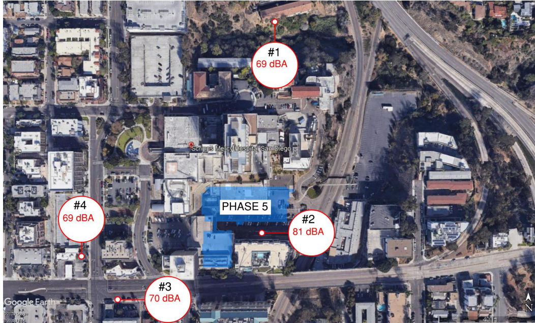
Figure 11 - Hospital I and Hospital Support Building Construction phase - total sound levels during allowed construction hours, at four receiver locations for the construction period
