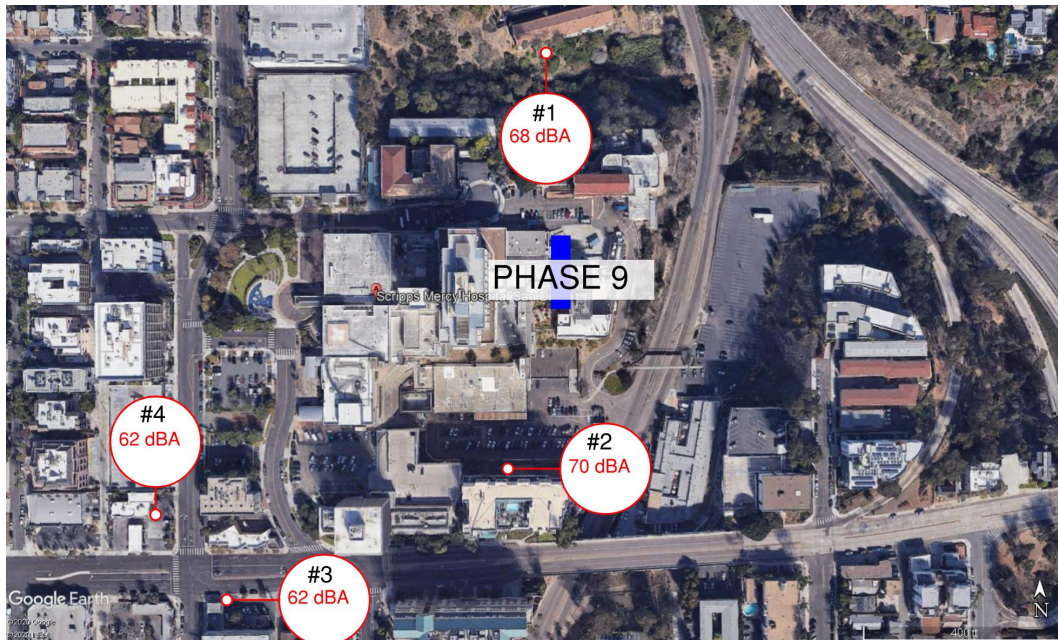
Figure 15 - CEP Expansion phase - total sound levels during allowed construction hours, at four receiver locations for the demolition period
