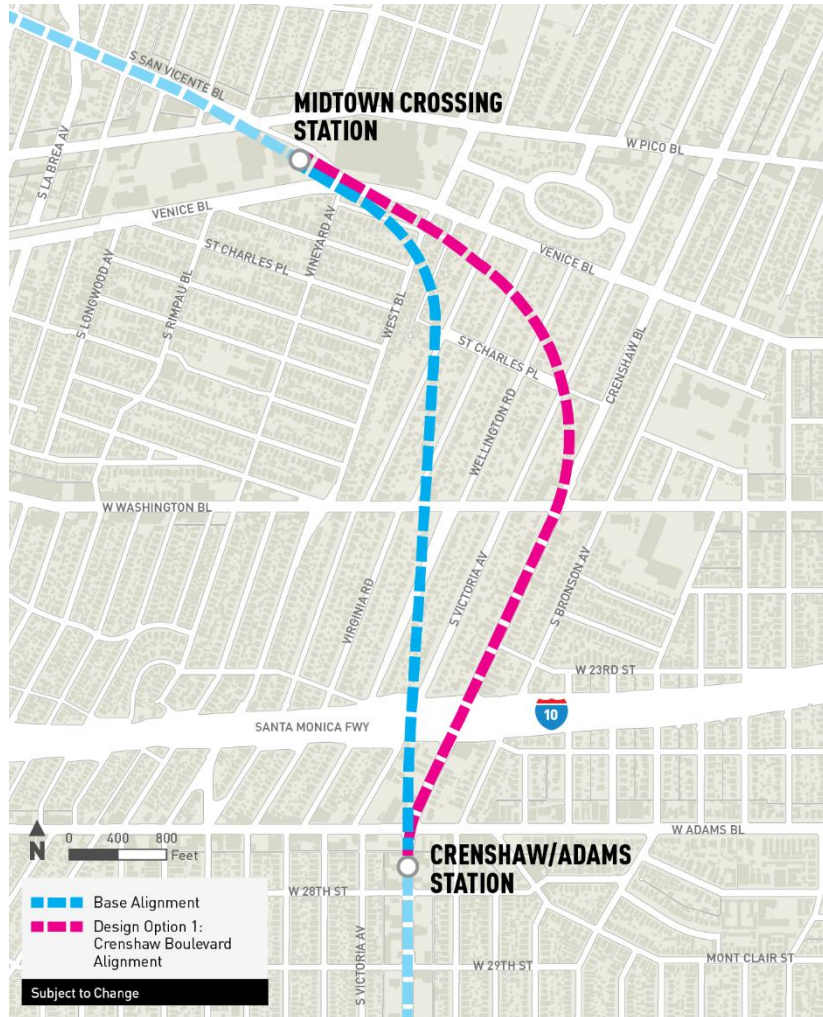
FIGURE 4-7. CRENSHAW/ADAMS TO MIDTOWN CROSSING ALIGNMENT DESIGN OPTIONS
