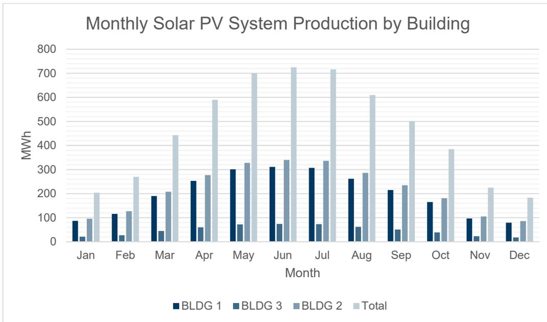
Figure 1: Estimated Monthly Production from PVWatts Simulation
