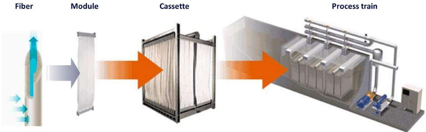
**Image 2-11b MBR Filtration Schematic**
