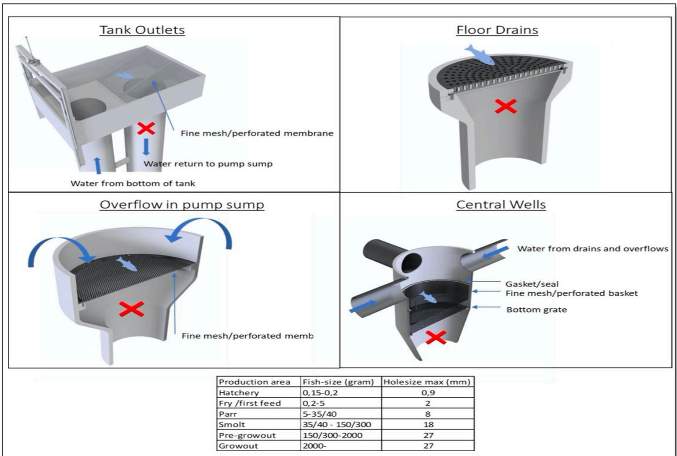
Image 2-10 Screen Overflow and Drain Designs with Hole Sizing (embedded table)
