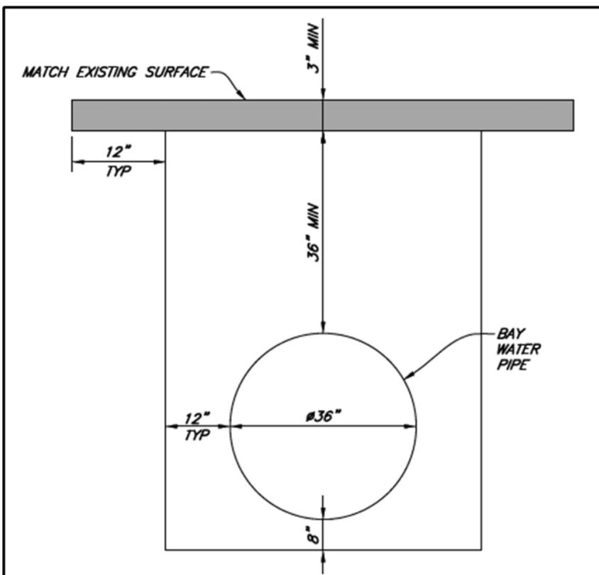
Image 2-21 Conceptual Trench Detail in the Area Where Only the 36" Bay Water Line Would Occur
