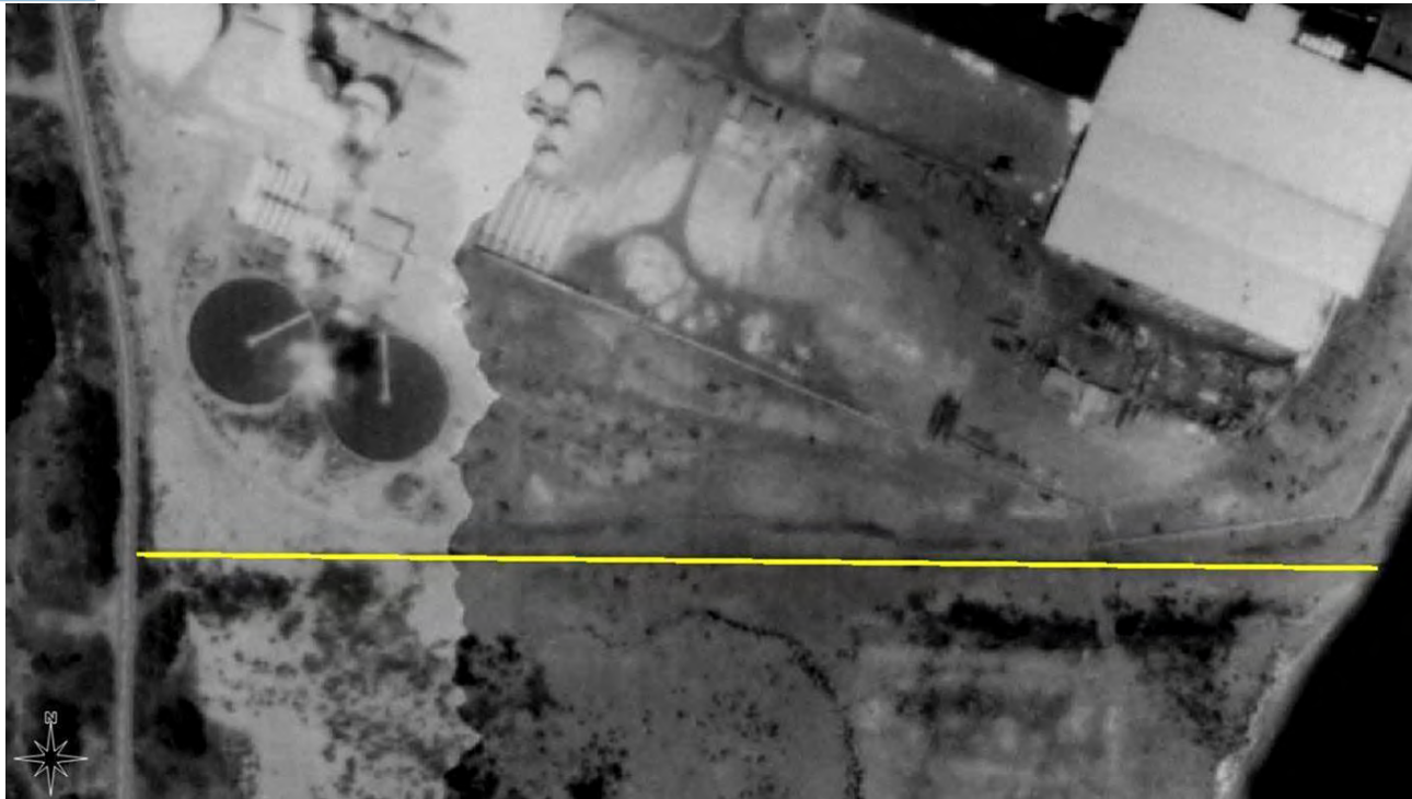
Figure 3. Imagery from 1970 shows additional grading on the west side of the site around the clarifiers that were installed during this period, and substantial vegetation removal south of the current fence line.
