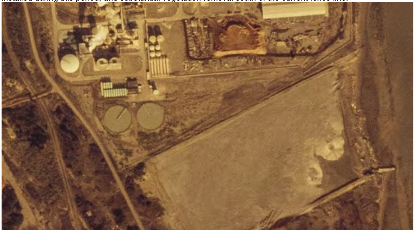
Figure 4. Imagery from 1973 shows clear formation of the berm along the southern fence line, and apparent hydraulic spreading of dredge spoils south of the berm within the study area.
